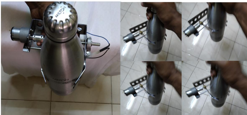
Figure 14. L.S.Gripper performance verification with Milton bottle
