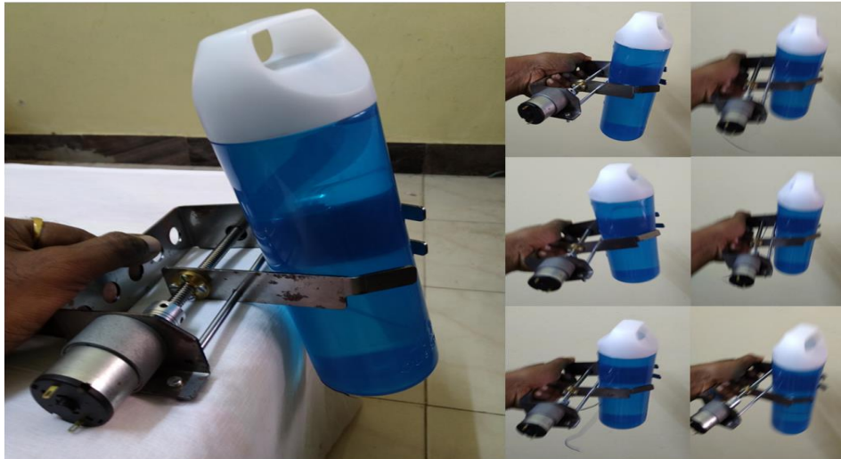
Figure 13. L.S.Gripper performance verification with Quechua bottle
