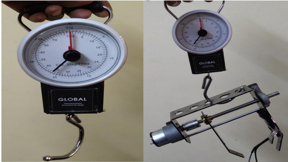
Figure 11. Analog weighing scale & gripper weight measurement
