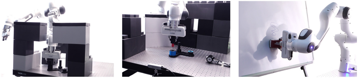
Fig. 6. (left) Obstacle navigation with joint velocity controller. (center) Vision-based peg-in-hole with velocity controlled robot. (right) White board wiping with force controlled robot.
