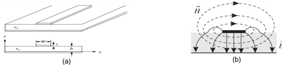
Figure 3. Microstrip Structure (a) Geometry, (b) TEM Field
