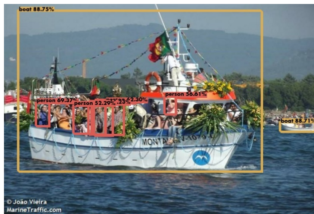
Figure 16: Output of the first round of experiments on MarineTraffic unseen imagery performing multi-class identification (e.g., instances of classes “person” and “boat”).
