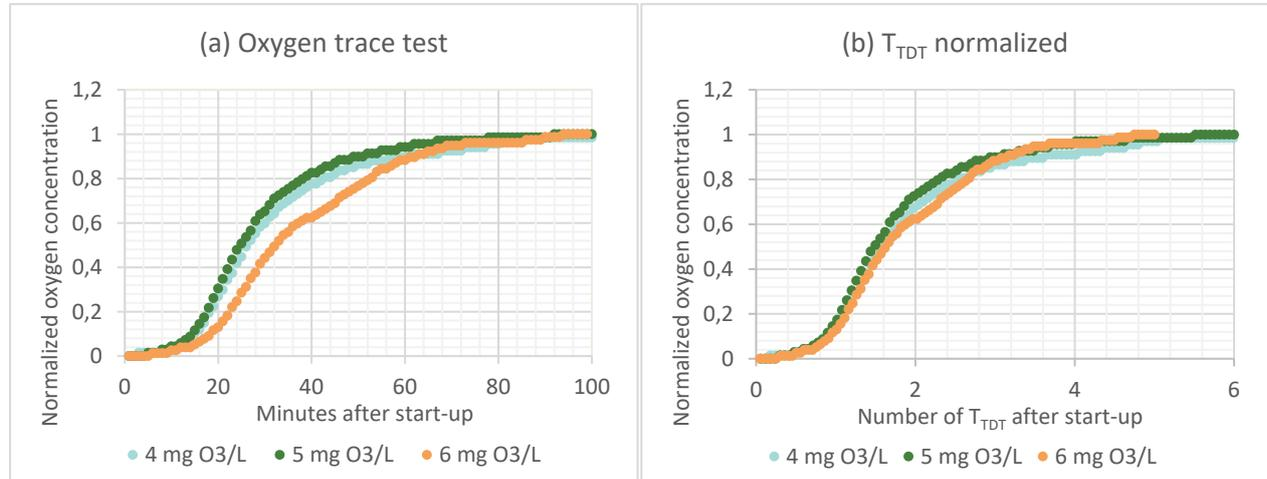
Figure 11: Normalized oxygen concentration in the water at the outlet of the ozone reactor after start-up of ozone production with the ozone doses 4, 5 and 6 mg O<sub>3</sub>/L. In (a), the normalized oxygen concentration in S<sub>2</sub> are plotted against minutes after start-up of the ozone production. In (b), the x-axis are normalized on the  $T_{TDT}$  calculated for each test based on the water flow.
