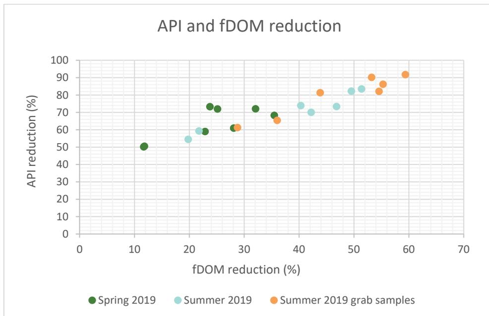
Figure 20: Correlation between the reduction of APIs and fluorescent dissolved organic matter (fDOM) measured in spring and summer full-scale sampling campaigns.
