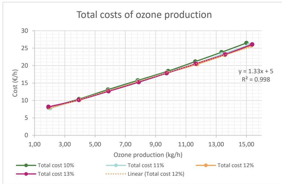
Figure 13: The total operational cost of the ozone reactor at different operational modes (ozone concentration in the gas) based on the prices for energy and LOX during the autumn 2018. The equation is a linear regression for the ozone concentration 12 %.
