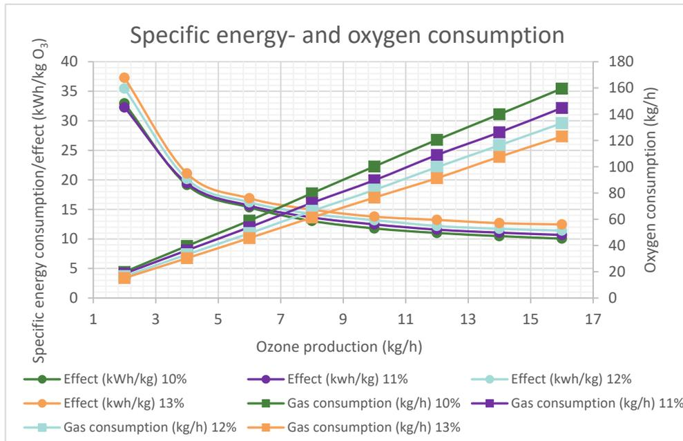
Figure 8: Specific energy consumption (effect) and oxygen consumption with increasing ozone production.
