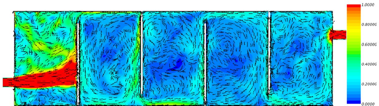
Figure 9: The first CFD flow simulation with the reactor volume distributed in five equally sized compartments. The arrows are showing the direction of the flow. The colour represents the velocity where red is the highest velocity and dark blue represents zero velocity.
