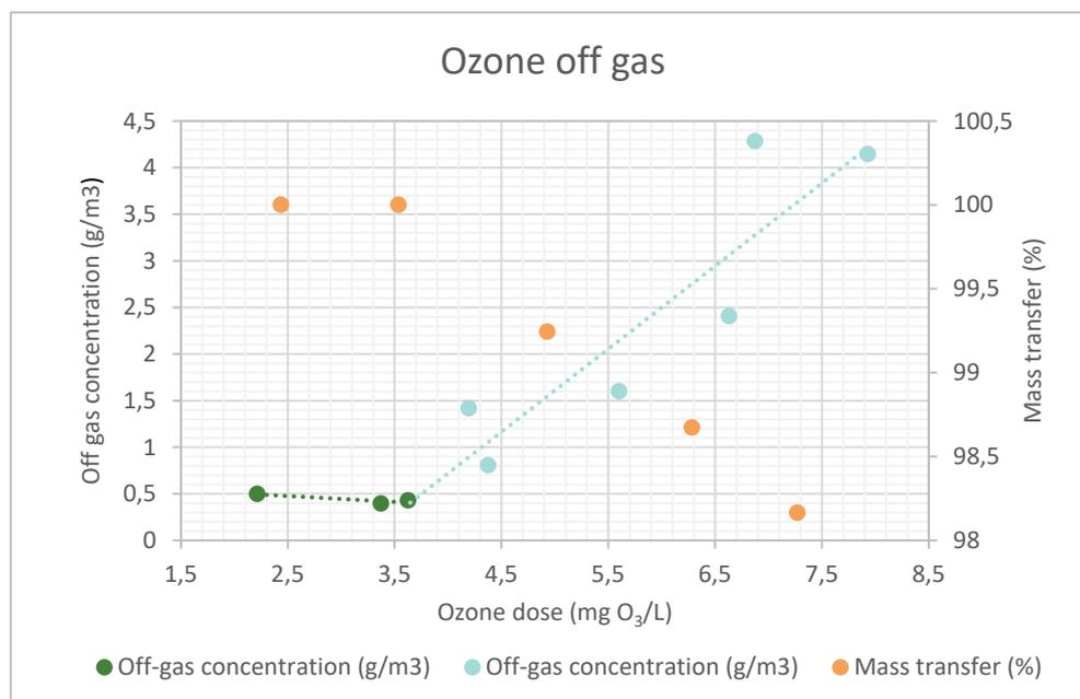
Figure 14: Ozone off-gas concentration and mass transfer for different ozone doses.
