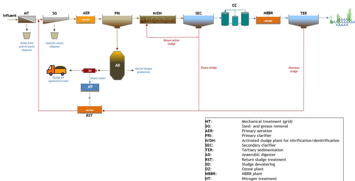
Figure 1: Overview of the WWTP Nykvarnsverket in Linköping.
