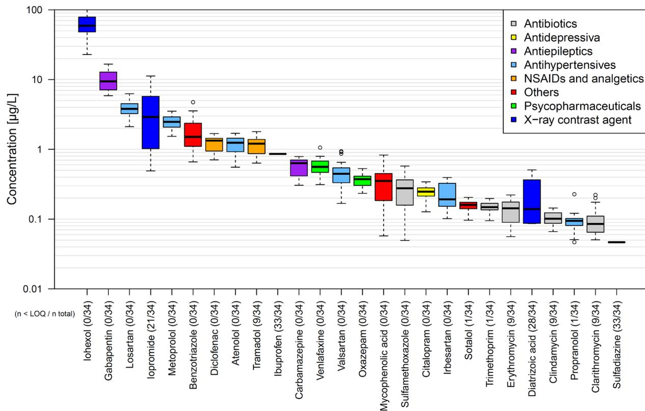
Figure 22: Concentrations of APIs measured in the secondary effluent (ozonation influent) in the full-scale sampling campaigns.
