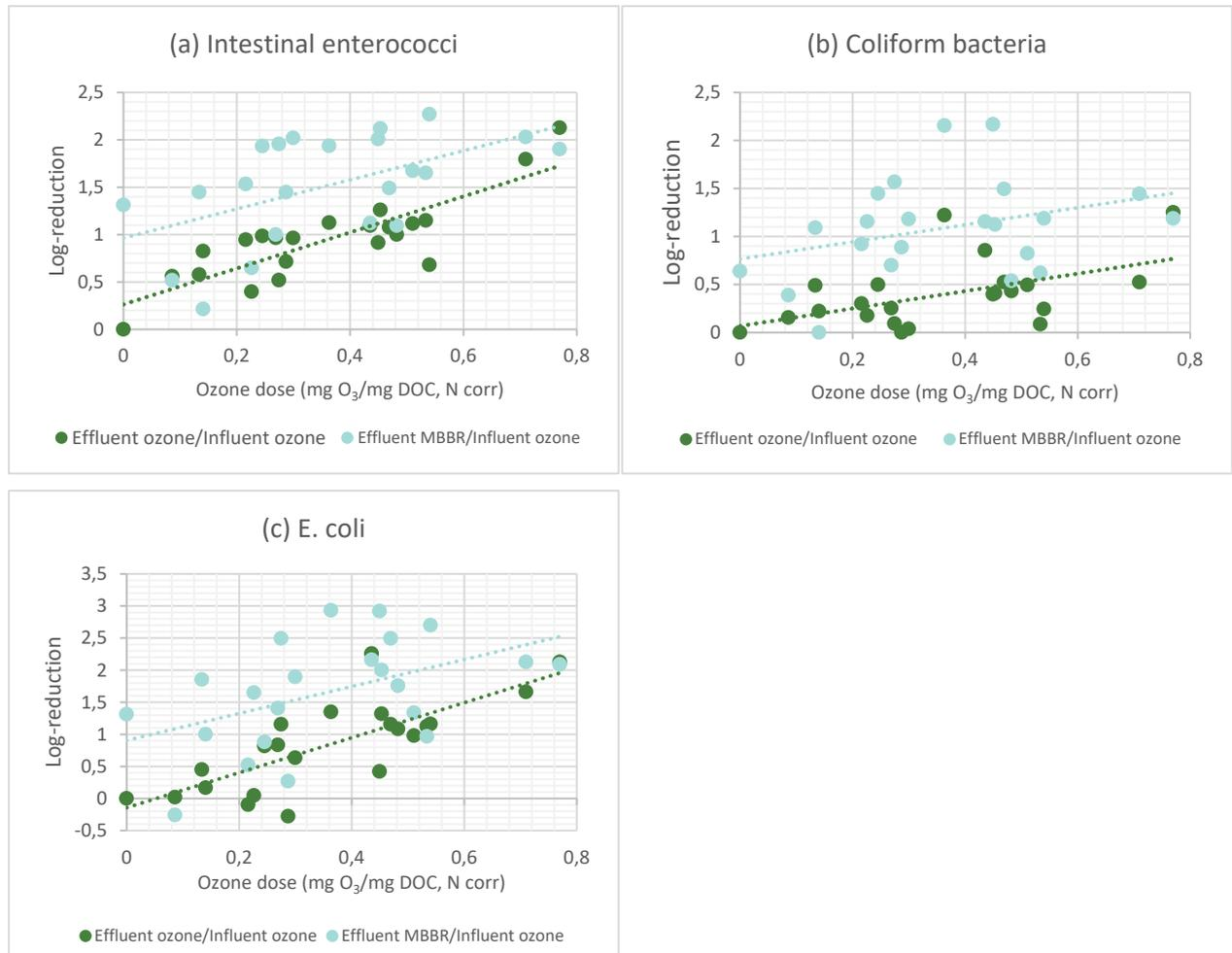
Figure 24: Bacteria reduction during ozonation and MBBR. The reduction is calculated as  $-\log_{10}(\text{out/in})$ .
