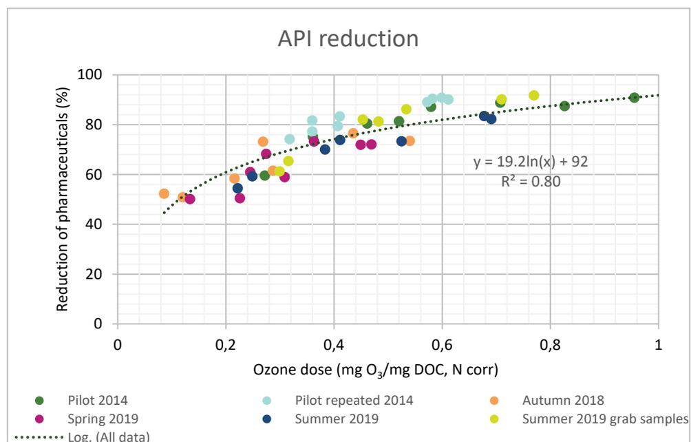
Figure 7: Average API reduction for different nitrite and DOC corrected ozone doses with an adjusted ozone dose for the first pilot tests. The dotted line and the equation represent the log-fit for all the data (both pilot and full-scale).
