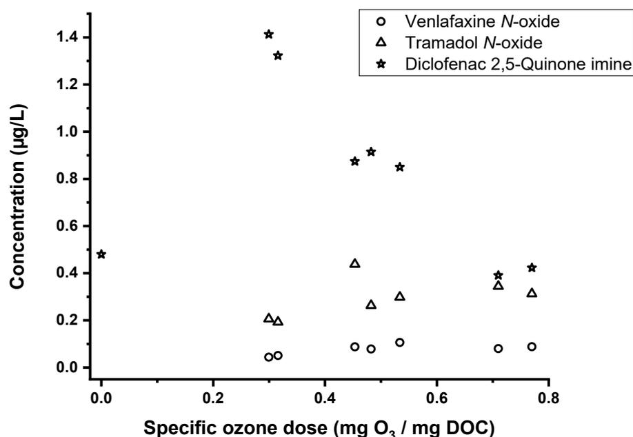
Figure 25: Concentration of N-oxide of tramadol and venlafaxine and Diclofenac 2,5-Quinone imine in the ozonation effluent.
