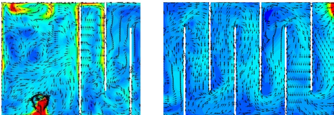
Figure 10: CFD simulation with the final reactor design. The figure is split in the first and the last part of the reactor.
