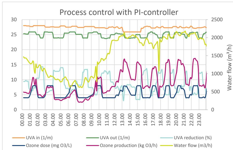
Figure 16: Ozone dose process control by a PI-controller using  $UVA_{254}$  reduction as process value.
