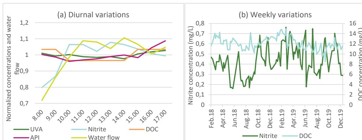
Figure 12: Diurnal and weekly variations in the secondary effluent. (a) Normalized concentrations of APIs, nitrite and DOC in the secondary effluent for grab samples collected before and after ozonation every hour between 8:00–17:00 and the water flow during one day. (b) Weekly variations of nitrite and DOC concentrations in the secondary effluent at WWTP Nykvarnsverket 2018-2019.
