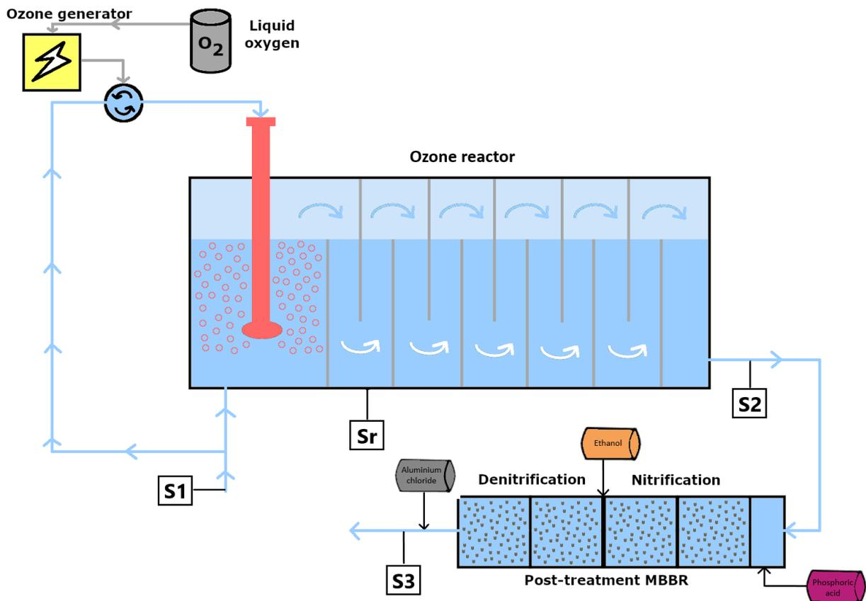
Figure 2: Overview of ozonation and MBBR process in Linköping. Four different sampling points are marked:  $S_1$  (before ozonation),  $S_2$  (after ozonation),  $S_3$  (after MBBR post-treatment) and  $S_r$  (first chamber of the ozone reactor).
