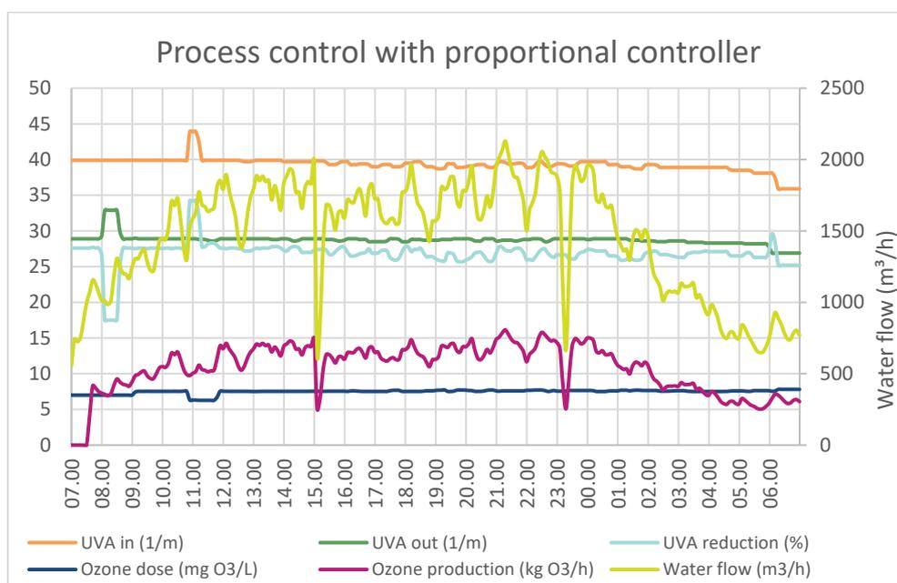
Figure 19: Ozone dose process control by a proportional controller with the settings in Figure 17.
