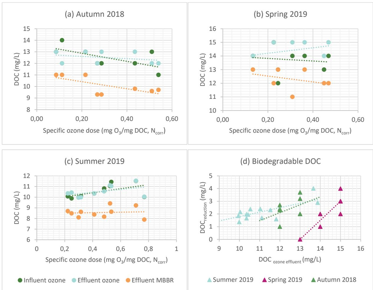
Figure 5: DOC concentrations at the ozonation influent, ozonation effluent, and MBBR effluent measured in the three sampling campaigns during autumn 2018 (a), spring 2019 (b) and summer 2019 (c). The specific ozone concentration on the X-axis only relates to effluent ozone and effluent MBBR. In figure (d) the absolute reduction of DOC concentration by the MBBR process is plotted against the DOC concentration at the ozonation effluent.
