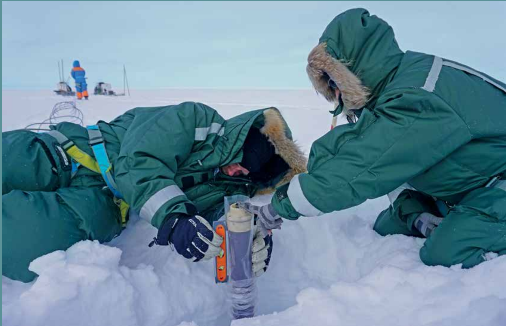
Installing a vertical magnetometer at the EastGRIP field camp on the Greenland Ice Sheet. Photo: Maaike Weerdesteijn.
