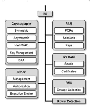
Figure 2, an overview of the TCG's TPM Architecture (image from [7]).
