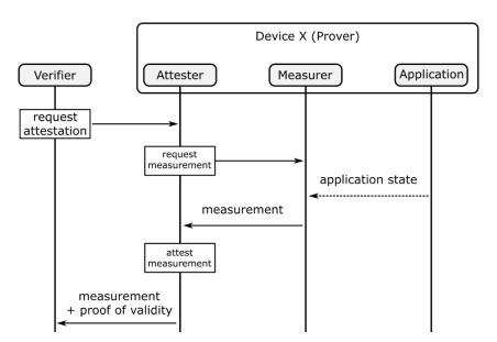
Figure 1, essential components of remote attestation.
