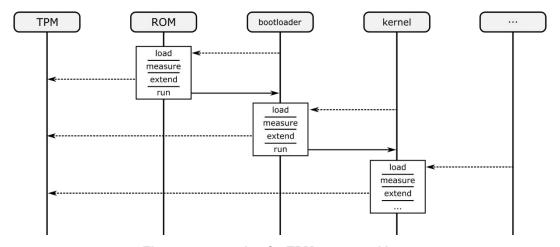
Figure 7, example of a TPM measured boot.
