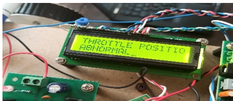
Fig 5. Abnormal throttle position indication
