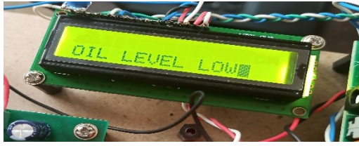
Fig 4. Low oil level indication
