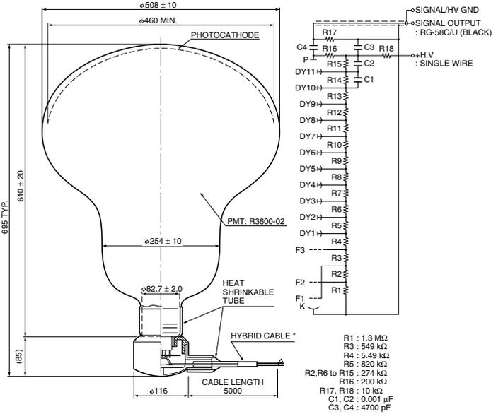
\* HYBRID CABLE CONTAINS A SIGNAL CABLE AND HV WIRE WITH ADDITIONAL COVER.
