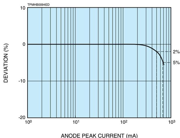
The special voltage distribution ratios are designed to achieve strong electric fields in the later stages of the electron multiplier. Some types are specified with these special voltage dividers.
