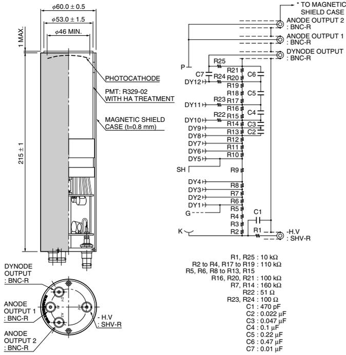
\* MAGNETIC SHIELD IS CONNECTED TO GND INSIDE OF THIS PRODUCT.
