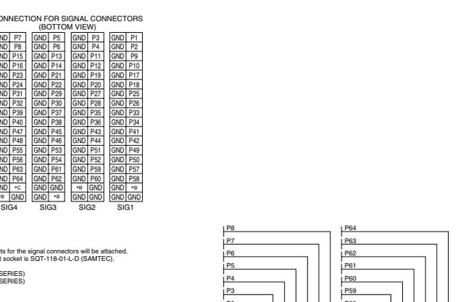
CONNECTION FOR SIGNAL CONNECTORS (BOTTOM VIEW)
