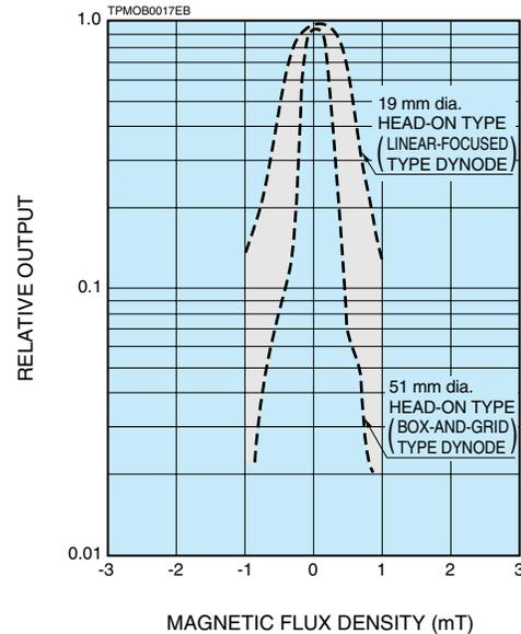
Figure 12: Edge Effect of Magnetic Shield Case
