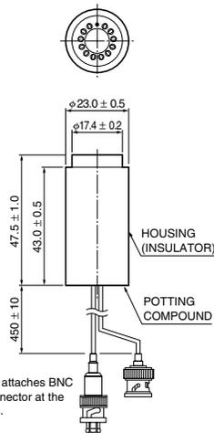
E974-17, -18 attaches BNC and SHV connector at the end of cables.
