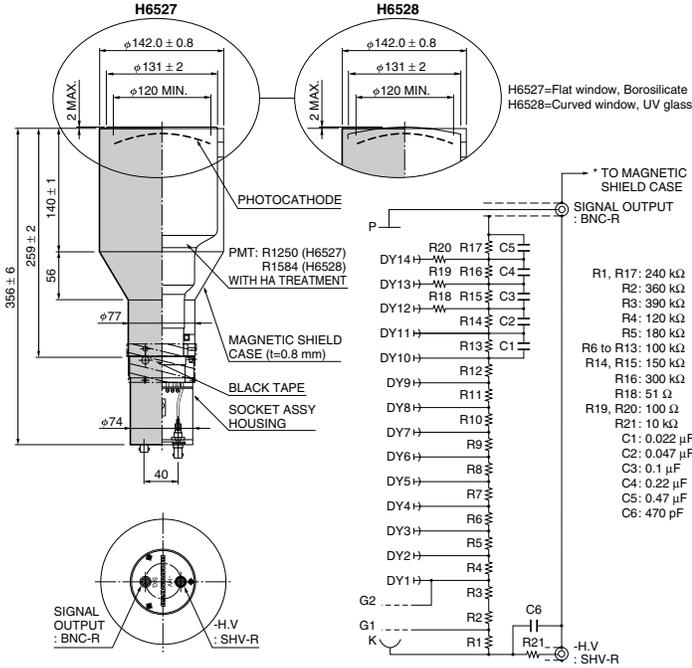
\* MAGNETIC SHIELD IS CONNECTED TO GND INSIDE OF THIS PRODUCT.
