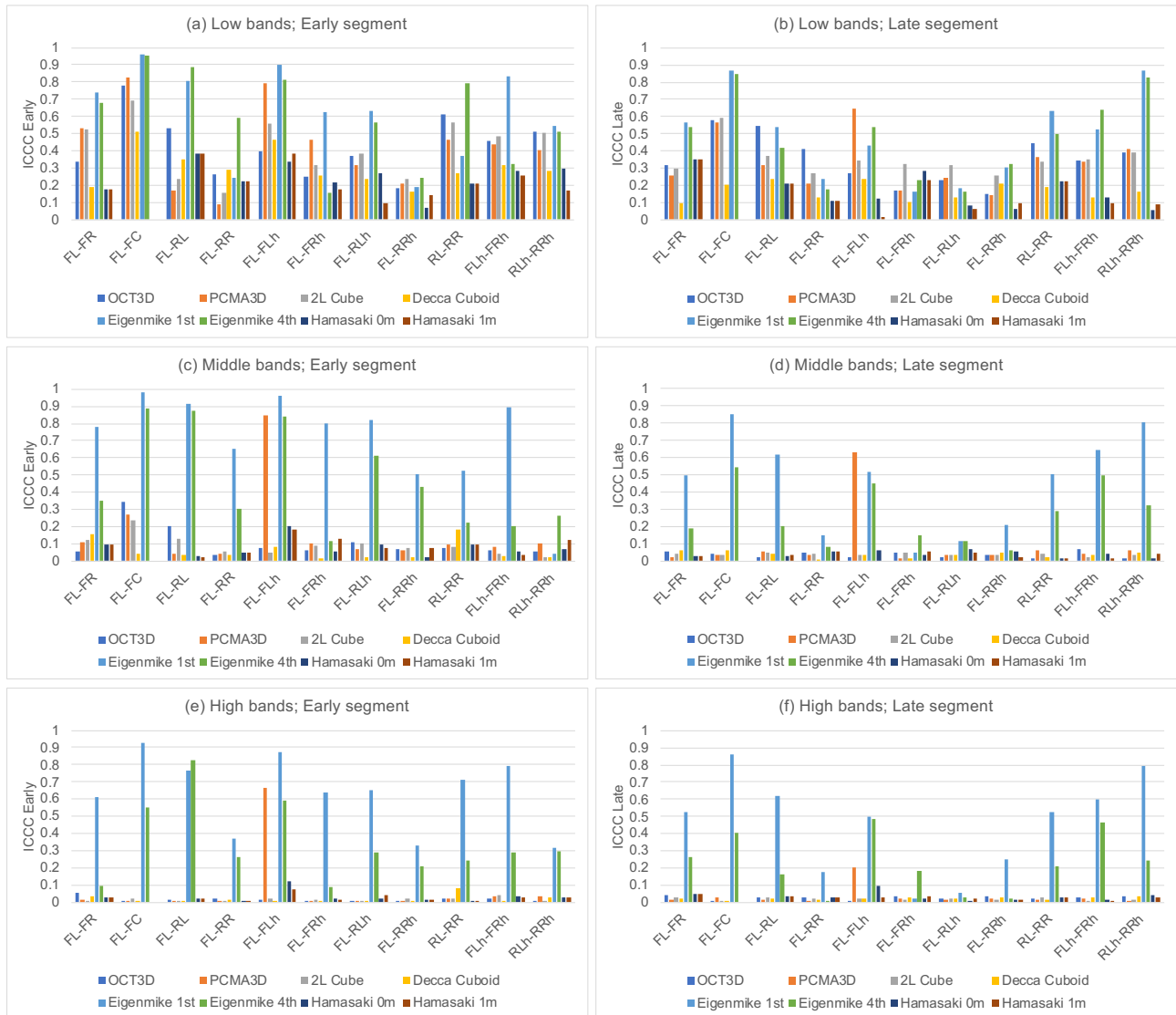
Fig. 10. Interchannel cross-correlation coefficients for various pairs of microphone signals.
