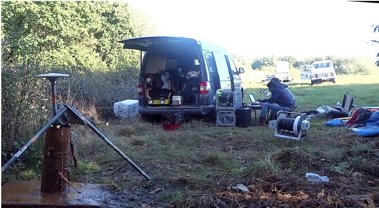
Figure 13. Temperature profile monitoring using DTS and flow measurement on study wellbore PZ-26 in Ploemeur-Brittany (October 2018).
