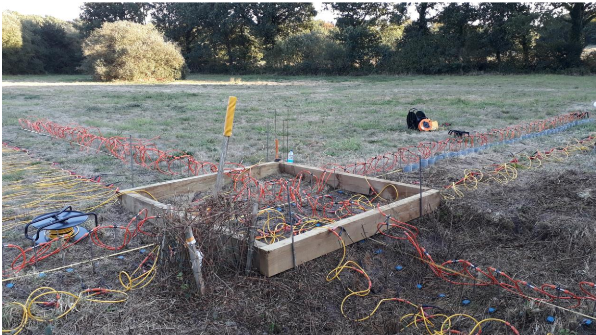
Figure 12. Acquisition set-up for the infiltration test at the Ploemeur Hydrological Observatory. The wood planks delimit the infiltration area.
