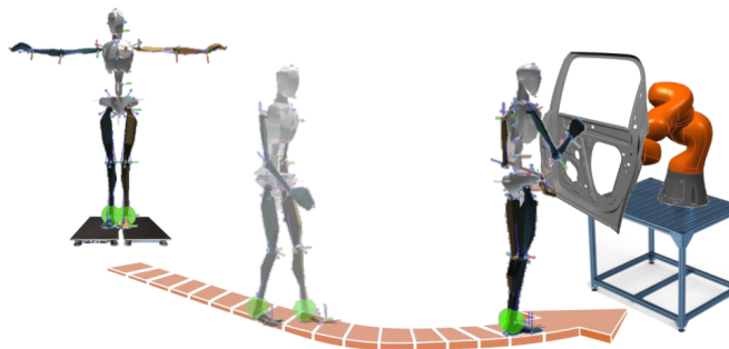
Fig. 1: Concept illustration of on-the-fly human model identification and ergonomics monitoring during work in industrial settings.
