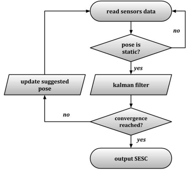
Fig. 4: Schematic block diagram of the estimation procedure.
