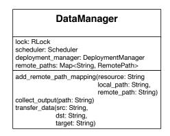
Figure 6: UML class diagram for the DataManager class.
