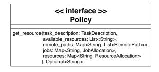
Figure 5: UML class diagram for the Policy interface.
