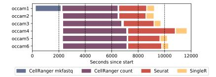
Figure 8: Execution timeline for the StreamFlow single-cell application on six Occam nodes, each allocated to both a CellRanger and an R environment containers.
