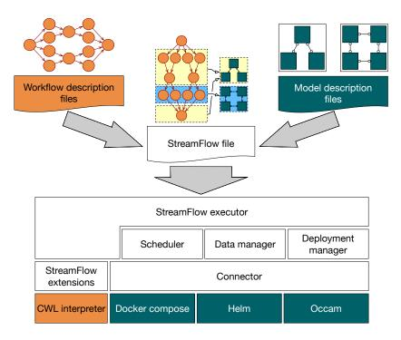
Figure 1: StreamFlow framework's logical stack. Coloured portions refer to existing technologies, while white ones are directly part of StreamFlow codebase. In particular, the orange area is related to the definition of the workflow's dependency graph, while the green area refers to the execution environments.
