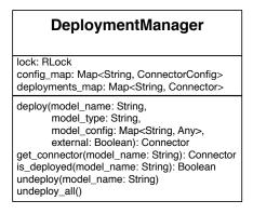
Figure 3: UML class diagram for the DeploymentManager class.
