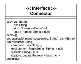
Figure 4: UML class diagram for the Connector interface.
