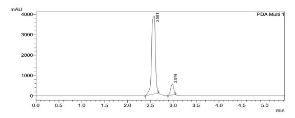
Figure 12: Chromatogram of standard solution of TEN at 100µg/ml and EMT 800µg/ml.
