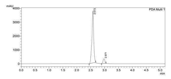
Figure 10: Chromatogram of standard solution of TEN at 60µg/ml and EMT 480µg/ml.
