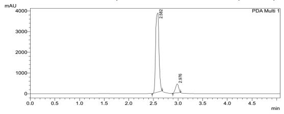
Figure 11: Chromatogram of standard solution of TEN at 80µg/ml and EMT 640µg/ml.
