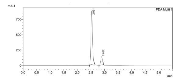
Figure 17: Robustness at mobile phase ratio 90:10.
