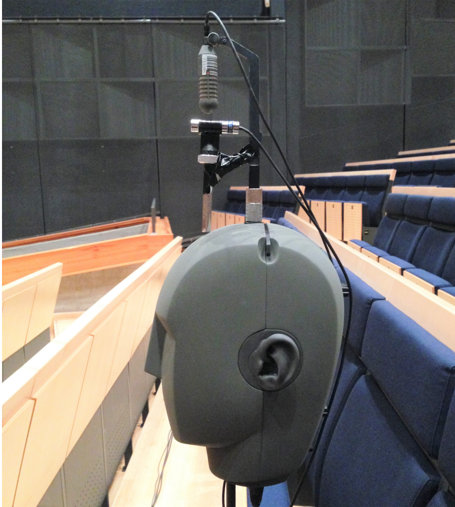
Figure 4.2: Binaural head with OmniFig8 array mounted on top (in KH).
