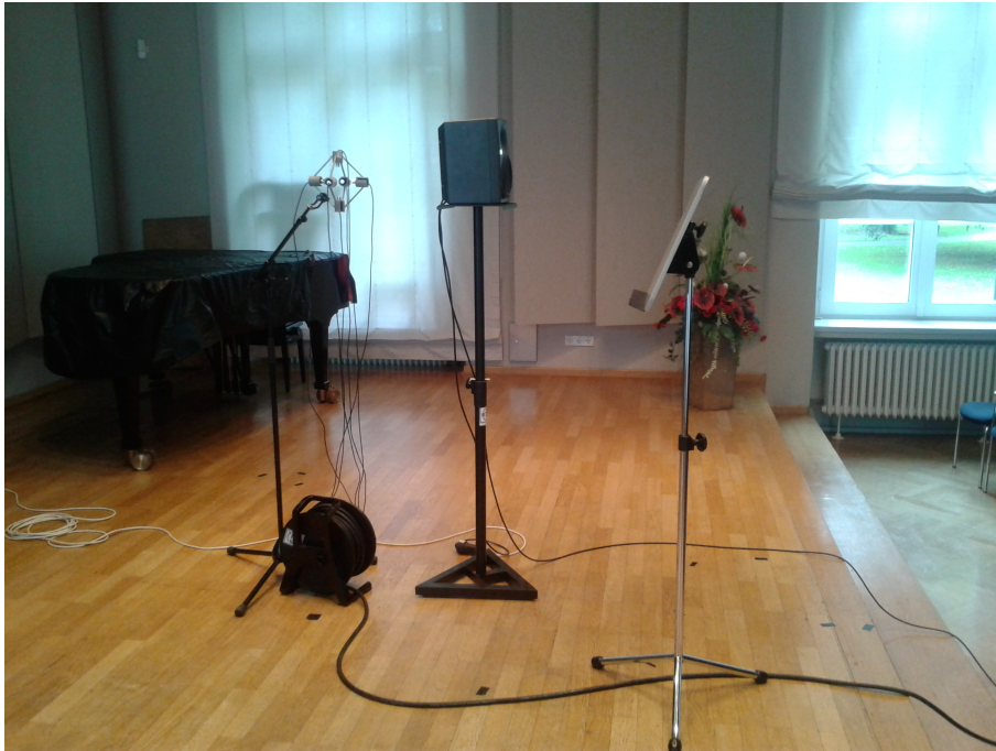
Figure 5.1: Exemplary stage measurement configuration of Set A: single source (Neumann KH120), open array and music stand (in BS).
