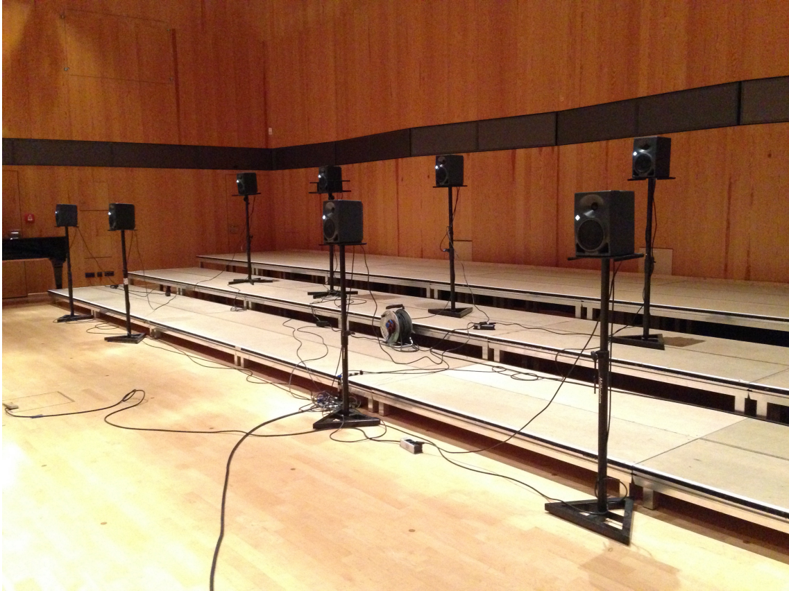
Figure 5.3: Loudspeaker orchestra (8 sources) on stage at KH. The MAP array used for WFS and artificial reverberation can be seen mounted on the wall.
