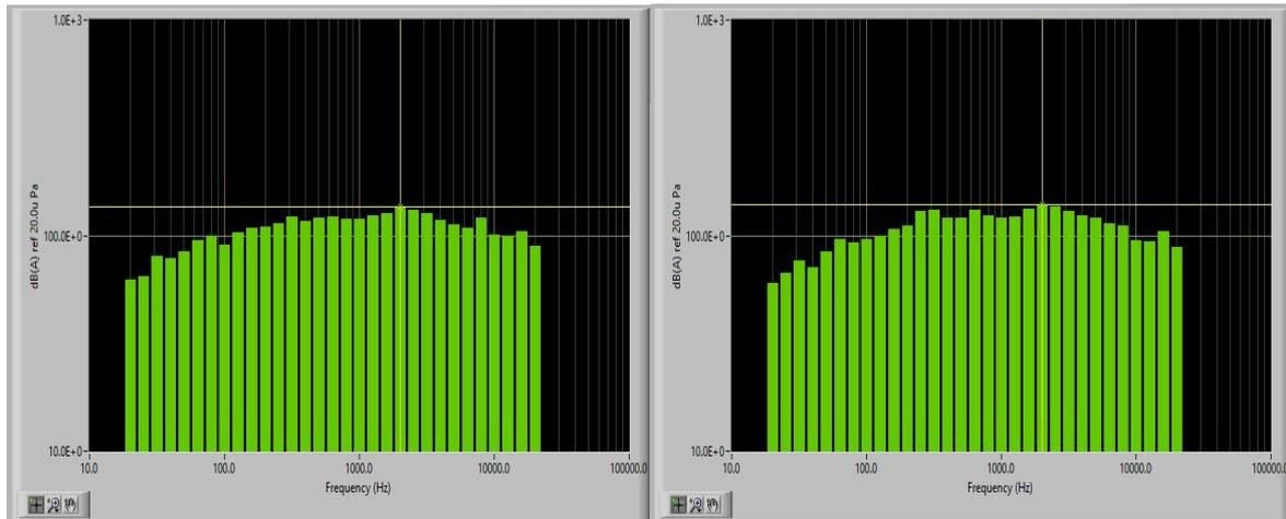
**Fig.11:-** Sound signal with 1/3 octave for healthy and faulty gears at the speed of 400rpm and load 5kg.
