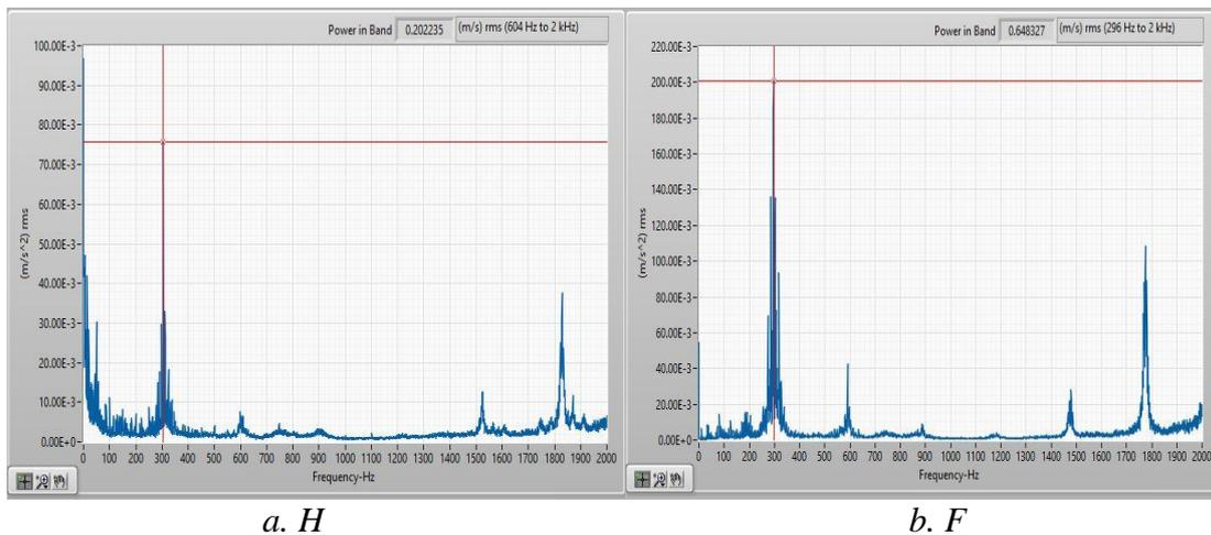
**Fig.8:-FFT Signals of Healthy and Faulty Gears at Speed of 400RPM and 5KG Load.**
