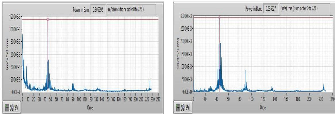
**Fig.10:-** Order Signal for Healthy and Faulty Gears at the Speed of 400RPM and Load 5KG.
