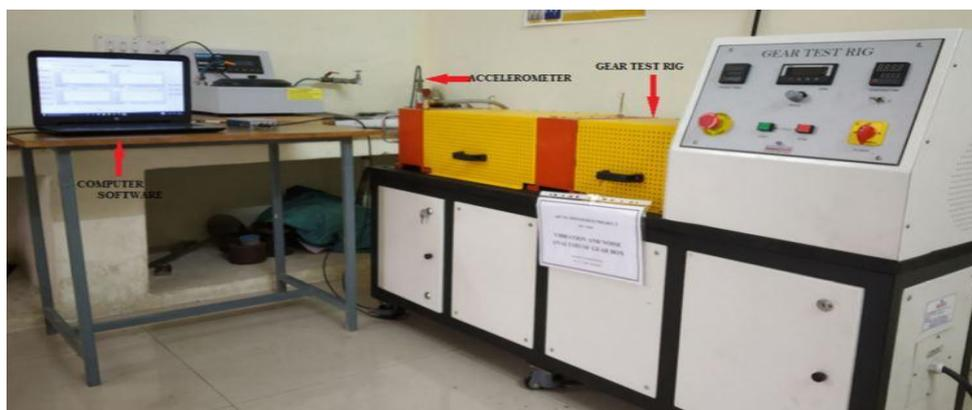
*Fig.2:-Experimental setup of gearbox test rig for vibration analysis.*
