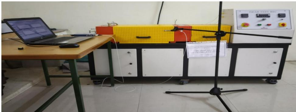
*Fig.1:-Experimental setup of gearbox test rig for noise analysis.*
