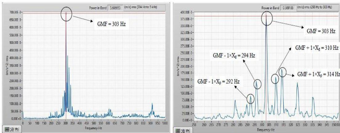
**Fig.9:- Zoomed FFT Signals of Healthy and Faulty Gears at Speed of 400RPM and 5KG Load Around GMF.**
