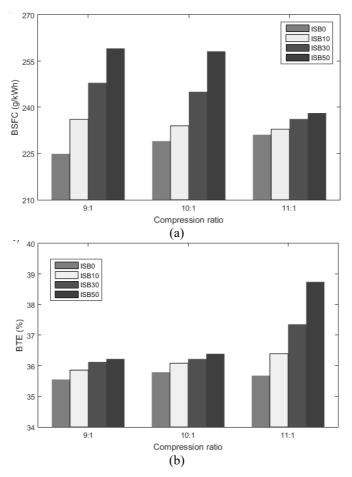
Figure 1. Variations of (a) BSFC and (b) BTE on CR, adapted from [88].
