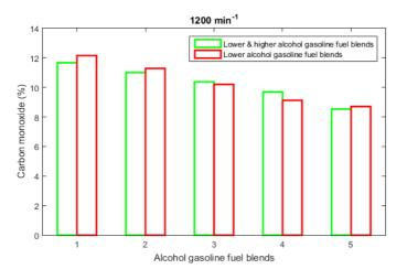
Figure 5. CO emission of various alcohol blends, adapted from [91].
