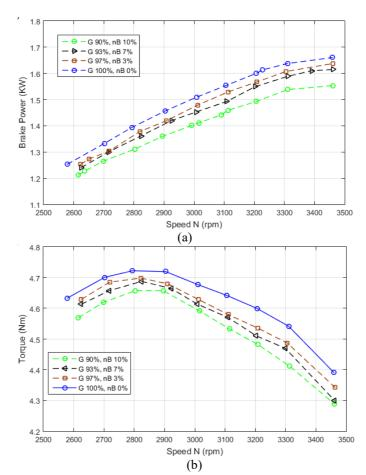
Figure 2. Power and torque against engine speed, adapted from [86].
