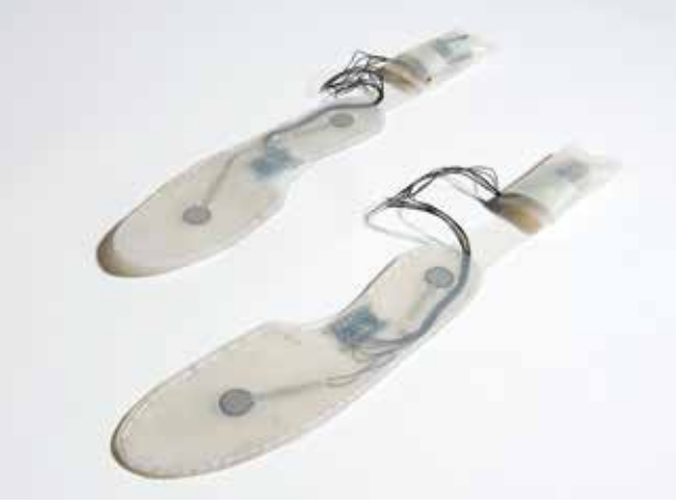
Audio Gait by Agnes Rosengren and Bernardo Aviles-Busch sonifies movements to aid the understanding of body balance while walking. The portable system is an easy learning aid for shin prosthetics training, which translates walking movements into auditory feedback.
