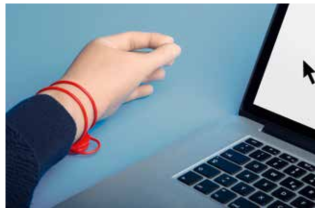
Shortcut by David Kaltenbach, Maximilian Mahal, and Lucas Rex is a customizable Human Interface Device (HID) for upper limb amputees. The bracelet detects sensory muscular impulses in the phantom hand, translating them into contactless and intuitive computer controlling.
