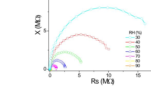
Complex impedance spectra of the mesoporous SnO<sub>2</sub> measured at different humidities and temperatures.
