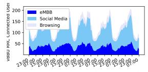
Figure 13: RRC connected users licenses per slice for a single vBBU instance in resource bound SLA setting with  $\alpha = [0, 50, 0], \beta = [75, 100, 100], \text{ and } R = 0.1.$
