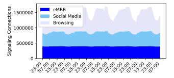
Figure 16: Signaling connections per slice at the vSDN controller for  $\alpha = [5 \times 10^5, 5 \times 10^5, 0]$ ,  $\beta = [10^6, 10^6, 10^{10}]$ , and R = 0.1.
