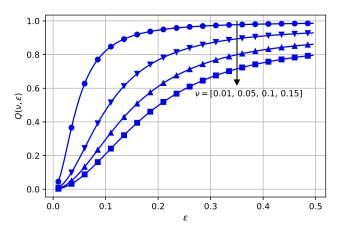
Figure 17: Reliable convergence probability vs.  $\varepsilon$  for R = 0.1,  $B_{\Delta} = 15.4$  and various violation rates  $\nu$ .
