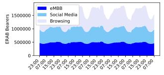
Figure 15: ERAB bearers per slice at the vDFE for  $\alpha = [5 \times 10^5, 5 \times 10^5, 0]$ ,  $\beta = [10^6, 10^6, 10^{10}]$ , and R = 0.1.
