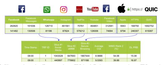
Figure 3: Slices creation and traffic aggregation at TRP level. Each row corresponds to a TRP at a given hour.
