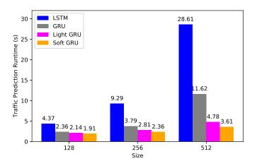
Figure 7: Prediction runtime for different recurrent networks architectures on a machine with Core i5-8500 CPU at 3 GHz and 16 GB RAM.
