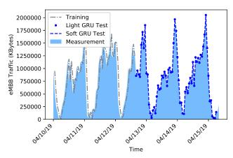
Figure 6: Predicted vs. measured traffics for eMBB slice at a TRP, with  $\epsilon = 0.7, 128 \times 1$  GRU.
