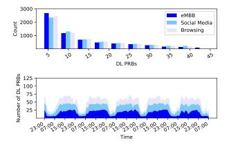
Figure 10: DL PRBs evolution and distribution per slice for SoA unconstrained resource allocation.
