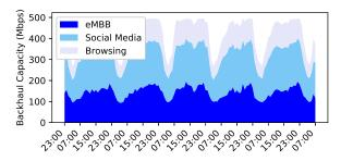
Figure 14: Backhaul capacity licenses per slice for a single vBBU instance with  $\alpha = [50, 100, 50]$ ,  $\beta = [150, 200, 150]$ , and R = 0.1.
