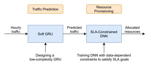
Figure 1: The main building blocks of the proposed data-driven network slicing resource allocation under SLA.
