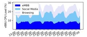
Figure 12: CPU consumption per slice for a single vBBU instance in resource bound SLA setting with  $\alpha = [0\%, 0\%, 0\%]$ ,  $\beta = [10\%, 15\%, 20\%]$ , and R = 0.1.
