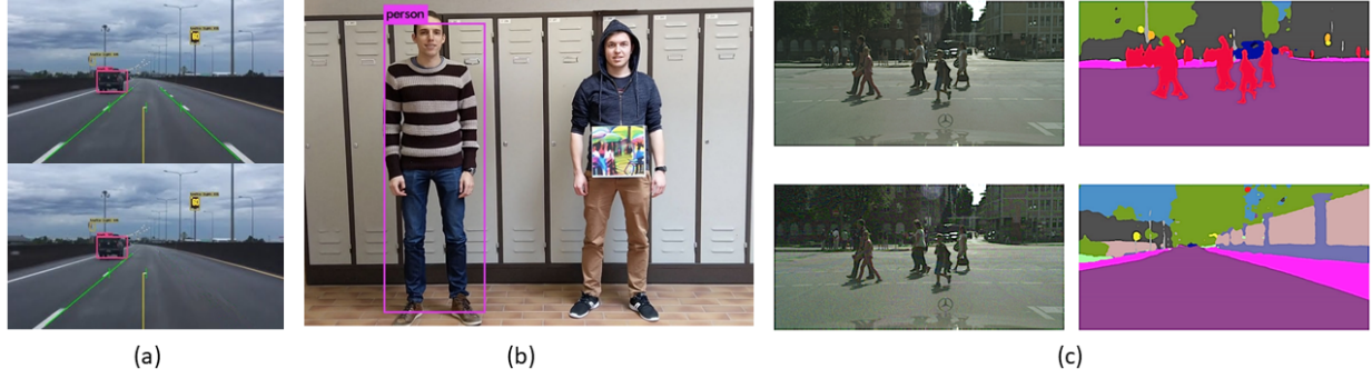
Figure 2: Attack scenarios on vehicle autopilot: (a) Lane lines removal can cause the car to steer in the wrong direction. (b) Adversarial patches can be used to mislead the visual detection module so that it does not detect pedestrians. (c) Adversarial attack on input image that causes the perception module to not detect the pedestrians.
