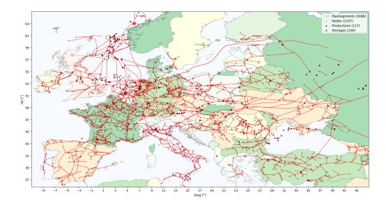
Figure 3.18: The pipelines, storage facilities and production sites of the EMap data set.
