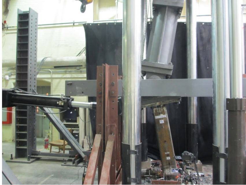
Figure 5.11 Deformed configuration of test setup
