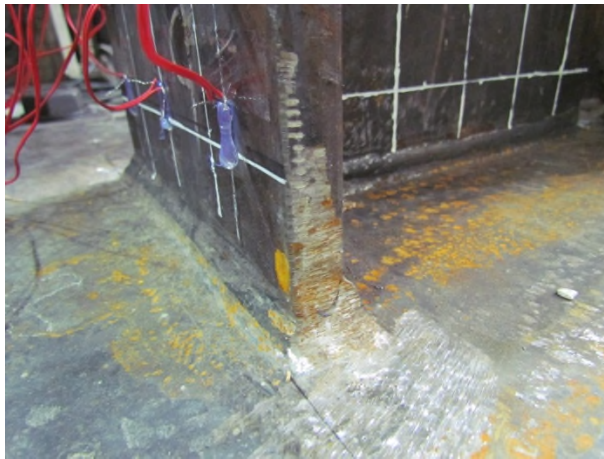
(b) Flange-to-base plate welding (W-8-34-S-C)
