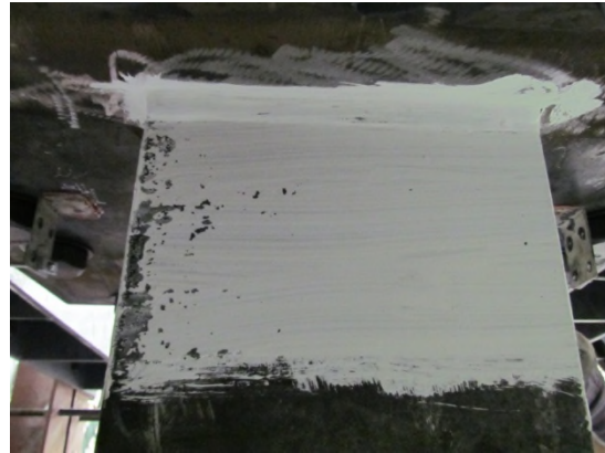
(h) Top end of north flange (White wash dropped due to the impact of brittle fracture.)
