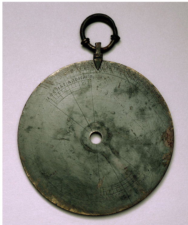
Figure 15. Byzantine exemplar dating from the 5th-6th century, diameter 110 mm. On the gnomonic face can be seen the cursor, which enables the dial to be set according to the latitude, and the pendant ring for keeping the instrument vertical in a chosen direction. On the angular sectors appear abbreviations in Greek letters of the Latin names of the months for each half year, January to June on the upper part, July to December on the lower. The read-off scale is lost. On the back are the latitudes of 36 cities and provinces. [credit: Trustees of the British Museum].
