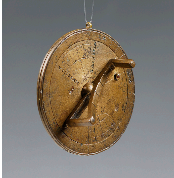
Figure 14. Roman exemplar found near Bratislava, dating from the 3rd century. The instrument is complete. Clearly visible are the mobile and curved read-off scale with its hour strokes, at the end of which is the gnomon. At the extremities of the date scale are the inscriptions VIII K. IAN and VIII K. IVL, which correspond to December 25 and June 24, the dates considered to be the winter and summer solstices in the Julian calendar.
