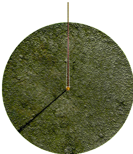
Figure 9. Photo of the rear face of the Berteaucourt-les-Dames disk. A gnomon was likely inserted in the hole to cast a shadow on the grid figuring on the other face of the disk. On the rear face shown here, a groove along the radius of the disk enables one to adjust it in the direction of the zenith.
