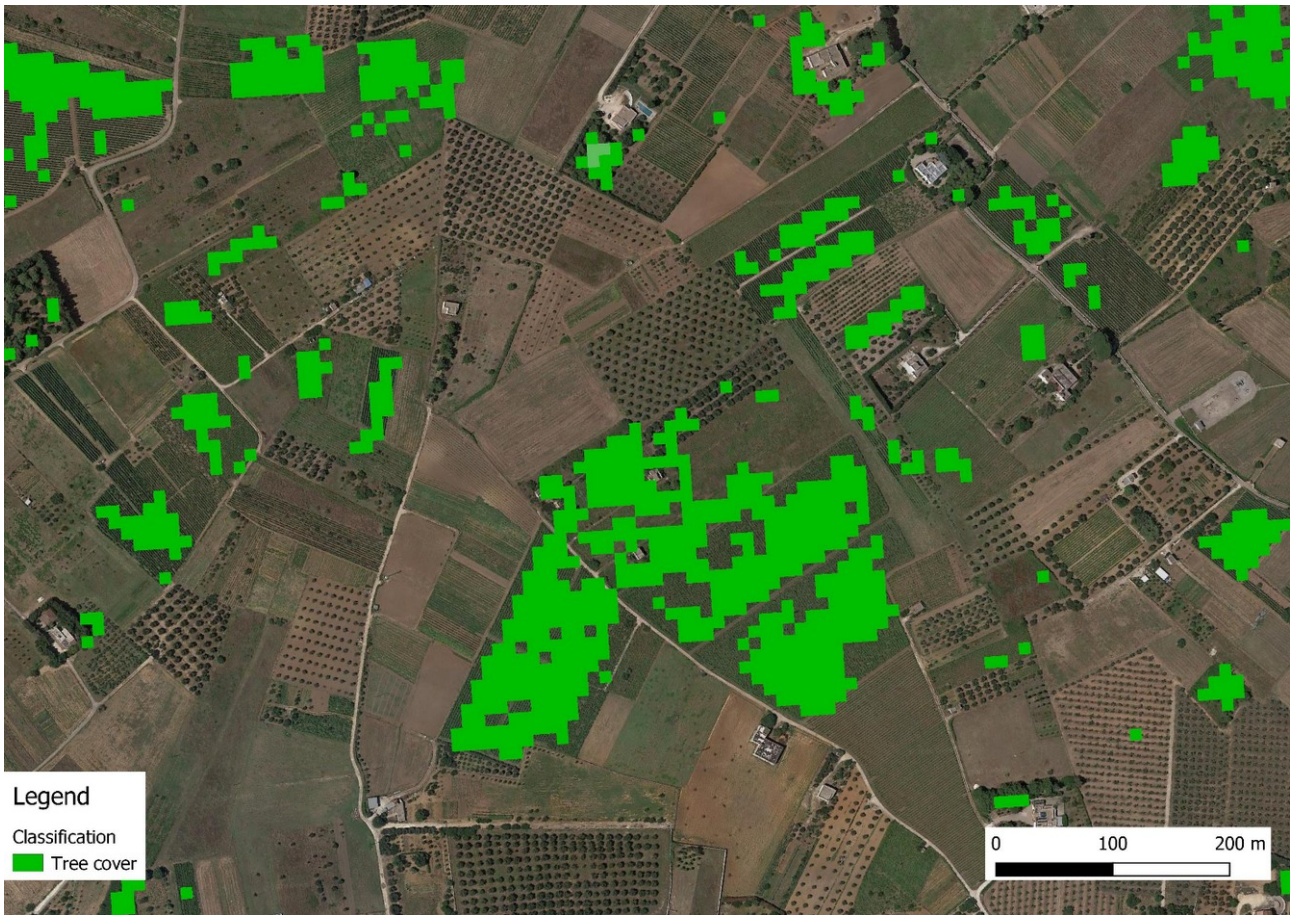
Figure 2: Example of tree cover classification (green) in Apulia (Google Earth image, 2017); olive trees are partially omitted.
