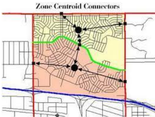
figure 14: zone centroid connection approach
