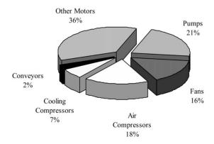
Figure 4. Disaggregation of electric motor use in the European Union (adapted from [40]).
