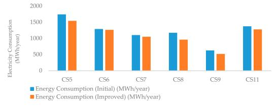
**Figure 6.** Electricity consumption for the initial and improved operation of the IWC (Average consumption cases).
