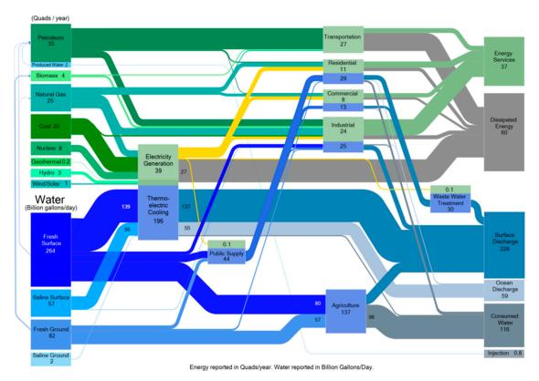
Figure 1. Sankey diagram for the water-energy nexus (adapted from [13]).
