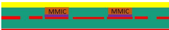
Figure 2: Embedded MMICs in a build-up structure consisting of Megtron 7N (green) and Ajinomoto-build-up film (yellow).
