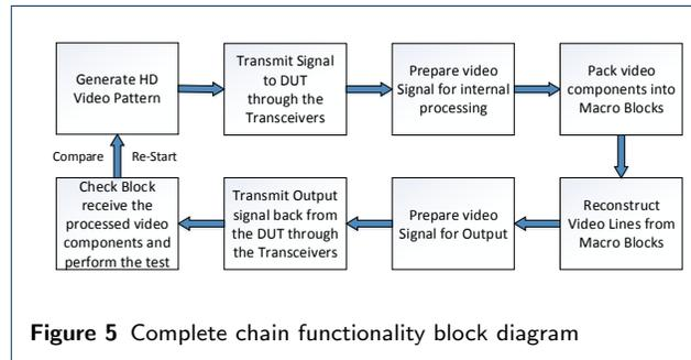
Figure 5 Complete chain functionality block diagram
