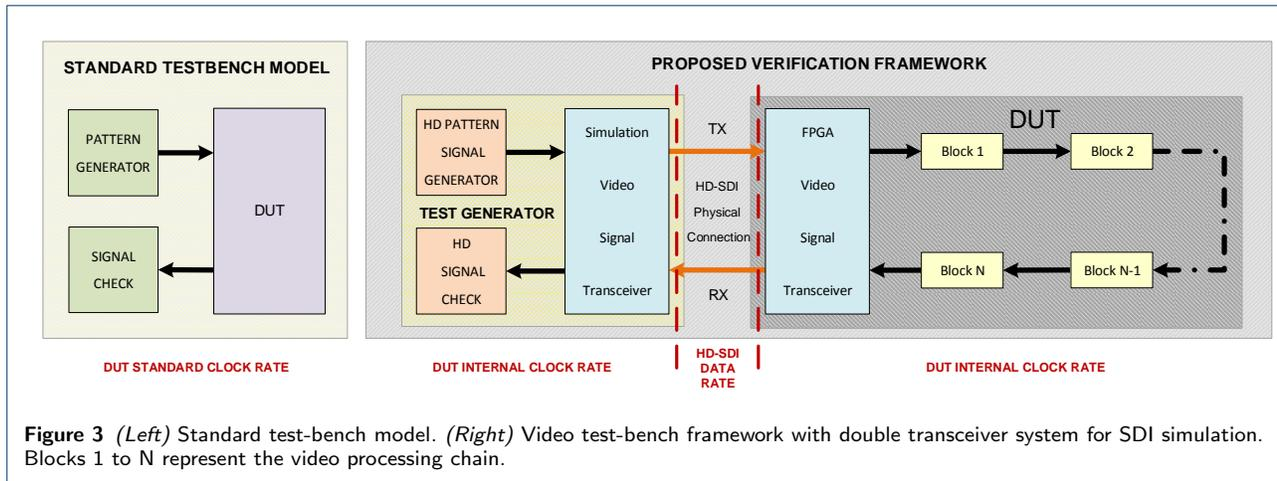
**Figure 3** (Left) Standard test-bench model. (Right) Video test-bench framework with double transceiver system for SDI simulation. Blocks 1 to N represent the video processing chain.
