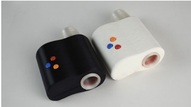
Spirotroller enhanced Game controller measuring the expiratory flow, 3d-printed, Bluetooth and USB, three buttons Direct use Actively developed
