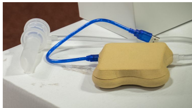
3D organic box Controller measuring the expiratory pressure, 3d-printed, USB, 1 LED Use with mouthpiece Actively developed
