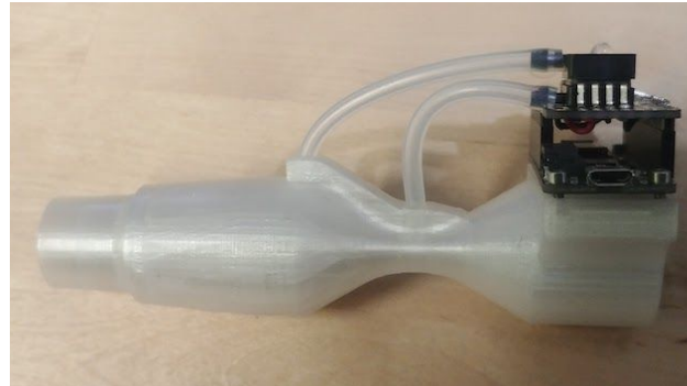
Spirotroller Game controller measuring the expiratory flow, 3d-printed, Bluetooth and USB, one button Direct use Prototyped
