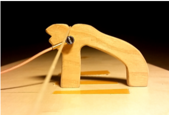
Fig. 2 Reproduced bridge with mounted pickup
