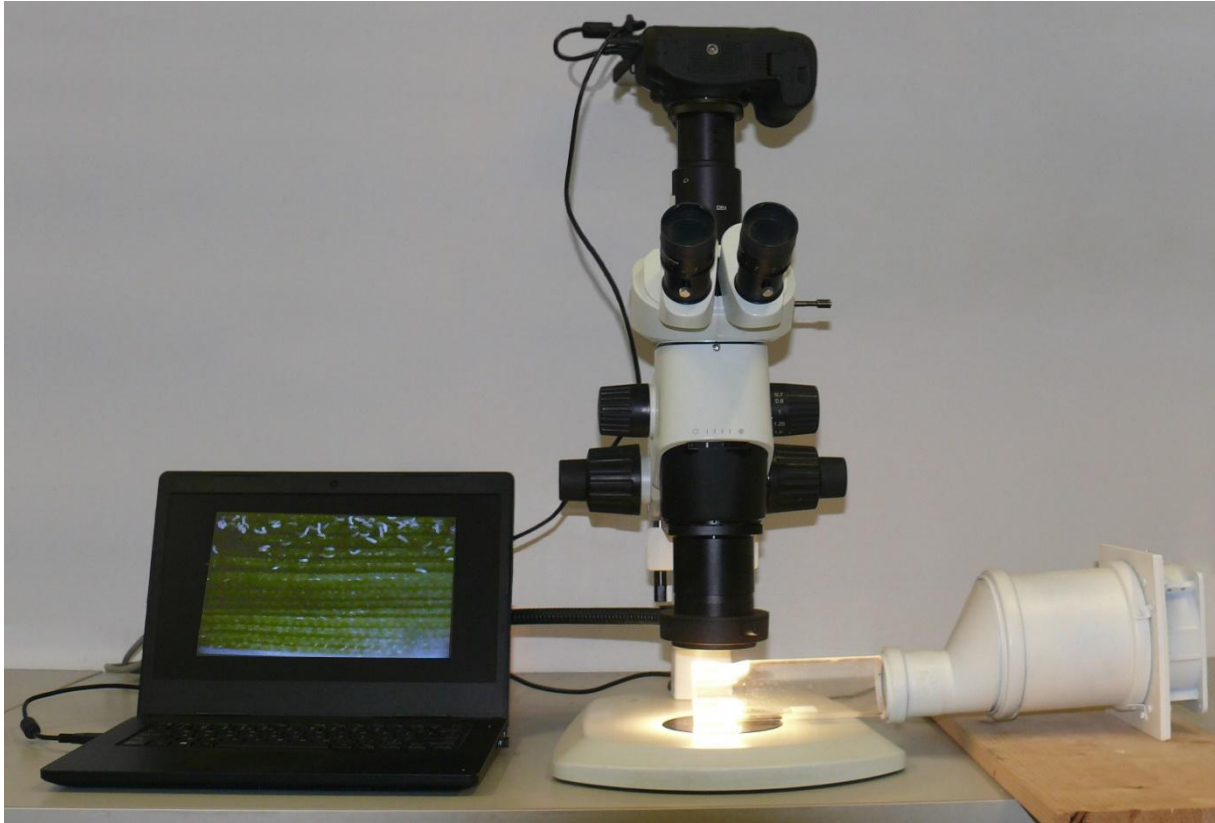
Fig. S3 Photo of the ‘departure’ tunnel used for direct observation and recording of departure events and dispersal-related behaviors in the presence of wind.
