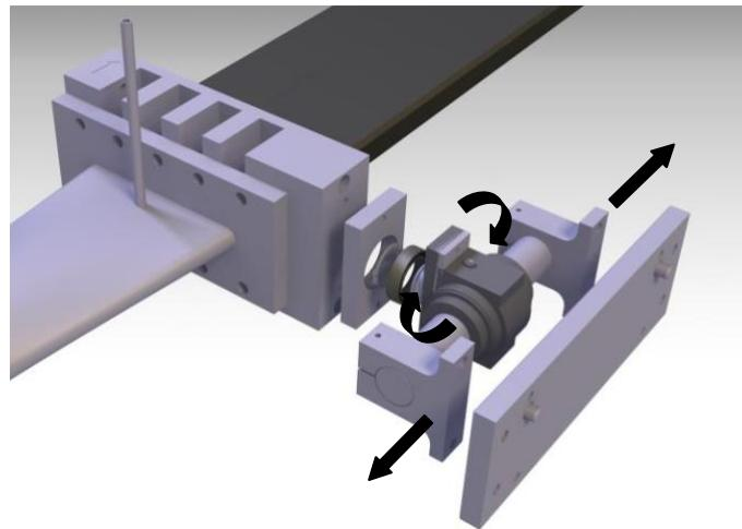
**Figure 2. Detail of the flexible mounting rig developed for this SiC receiver in order to cope with thermal expansion.**
