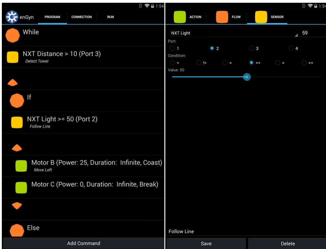
Figure 5. Preliminary Graphical User Interface (Programming Window, Command Window). Allows the user to create a list of commands using a dynamic interface that the robot can then perform.
