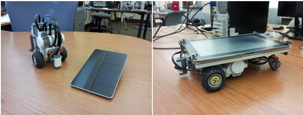
Figure 1. Setup (NXT and Android separate, NXT and Android integrated). Mobile device can be used with the robot separately to command remotely and display data to the user, or integrated to allow sensors from the mobile device to advance the robot's capabilities.
