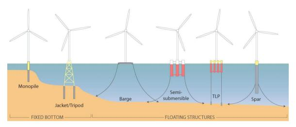
**Figure 1.1:** Common types of support structure technologies for bottom fixed and floating offshore wind turbines. [Source: Adapted from Principle Power]
