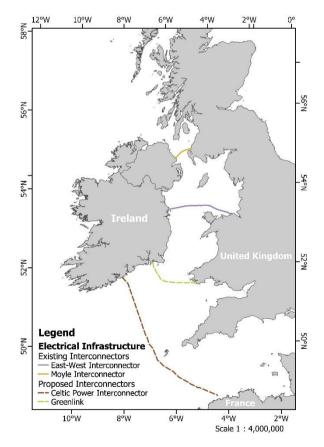
Figure 2.1: Existing and proposed electrical interconnectors in the island of Ireland (Scale 1: 4,000,000).
