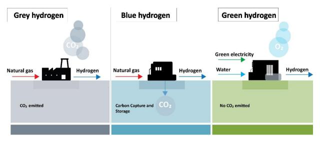
Figure 2.3: The differences between grey, blue and green hydrogen. (Adapted from: Gasunie).
