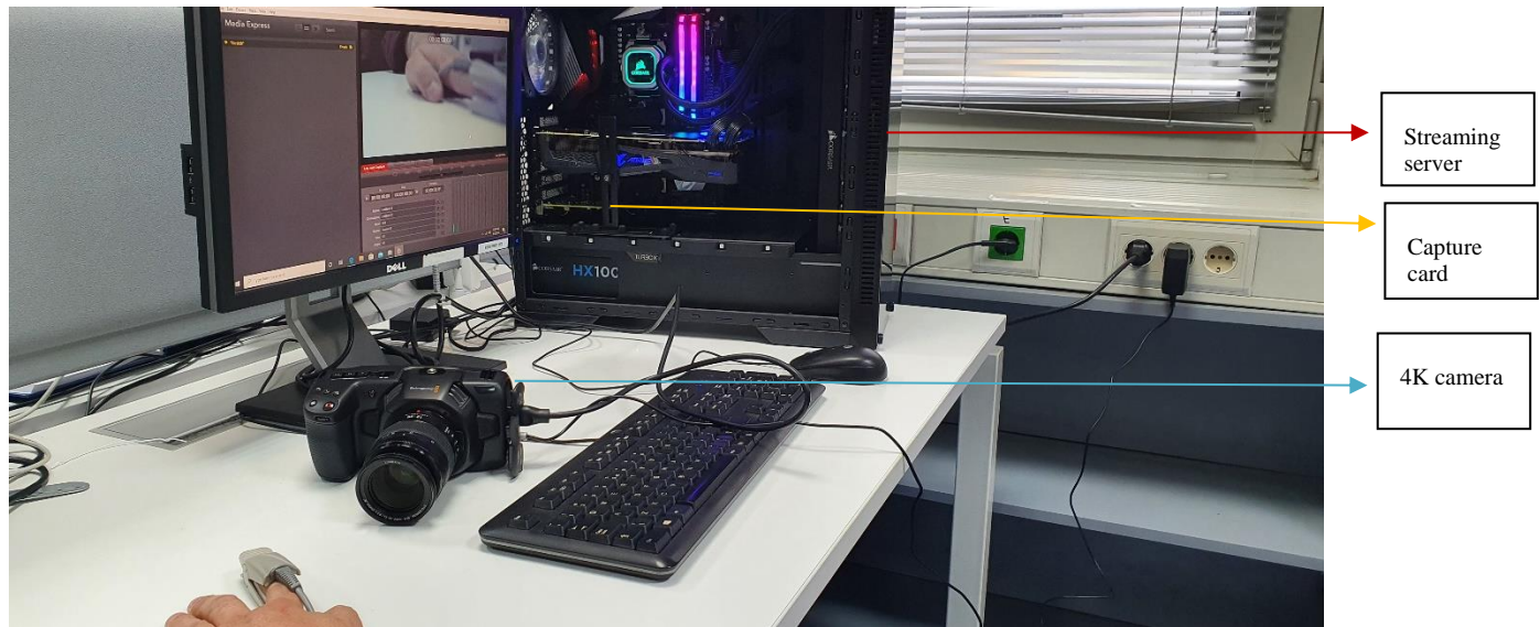
Figure 75: Smart City (Greece) UC5.4 - Use Case main components
