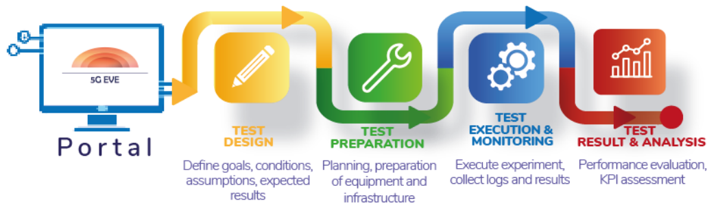
Figure 2: 5G EVE Portal - The 4-Step Process to 5G Validation
