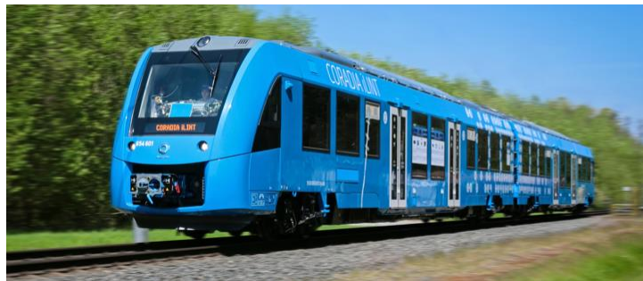
Figure 4-9: Coradia iLint hydrogen train receives approval for commercial operation in German railway networks [52]. It has a 1,000-kilometre range and can reach speeds of up to 140 kmh .
