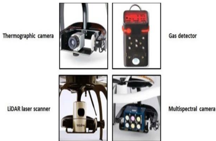
Figure 12. Examples of some Payload Types Required for IMTM UAS/RPAS Operations in Rail/Automotive
