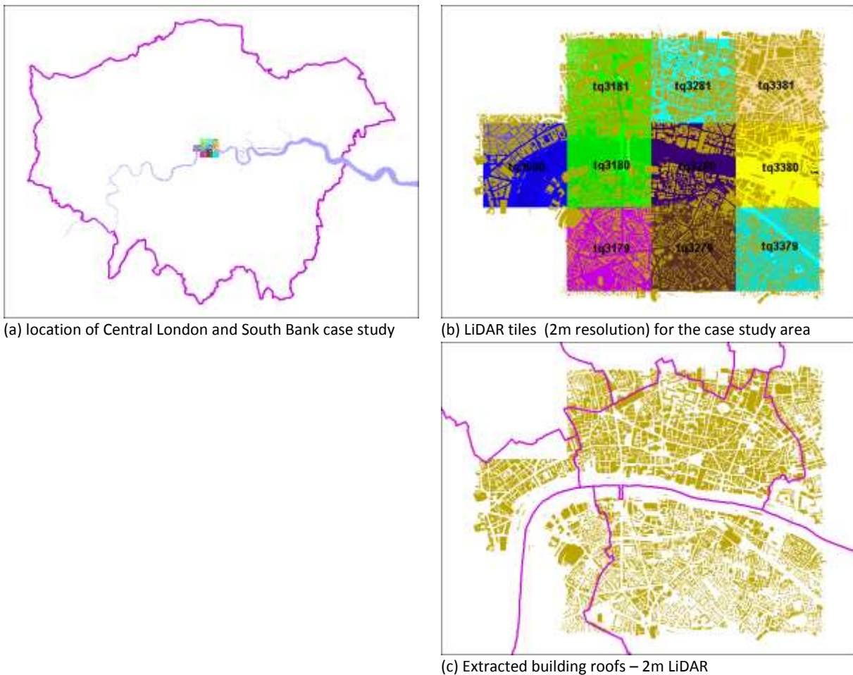
Figure 8.7: Location of Central London and South Bank case study, LiDAR tiles and building roofs.
