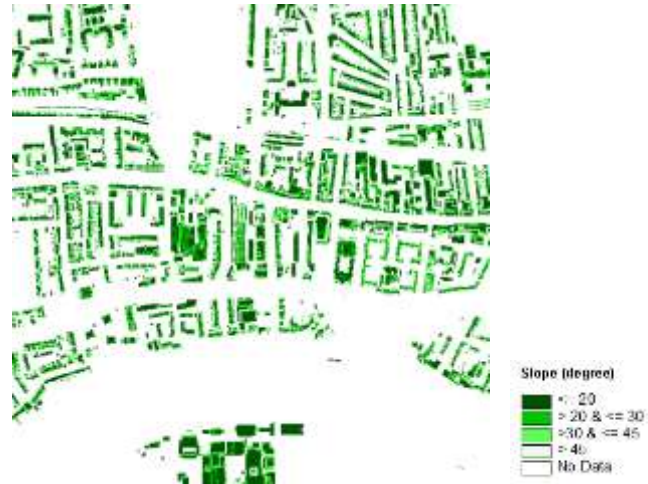
Figure 8.5: Slope of building roofs from 2m resolution LiDAR, Ravenscourt Park.
