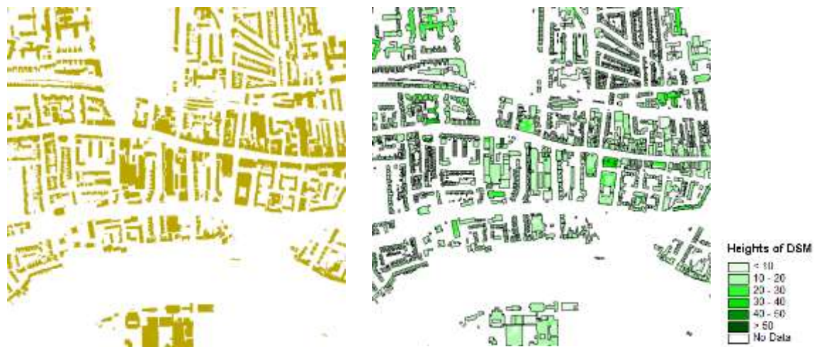
Figure 8.4: Cutting LiDAR DSM by rasterised building polygons to give 'buildings only' DSM, Ravenscourt Park.
