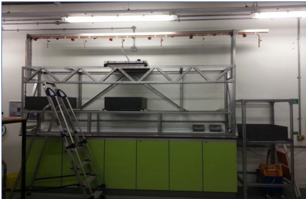
Figure 24. Rain simulator built as part of the TURAS project to test alternative materials for green roof construction under simulated storm event conditions
