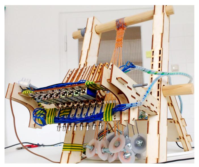
Figure 2: The Live Loom, a warp-weighted loom, with live-codeable heddles via solenoid actuators.
