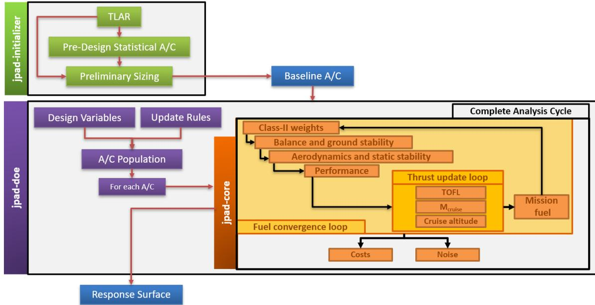
Fig. 6 Example of JPAD analysis workflow involving the *initializer*, the *core*, and the *doe* modules.
