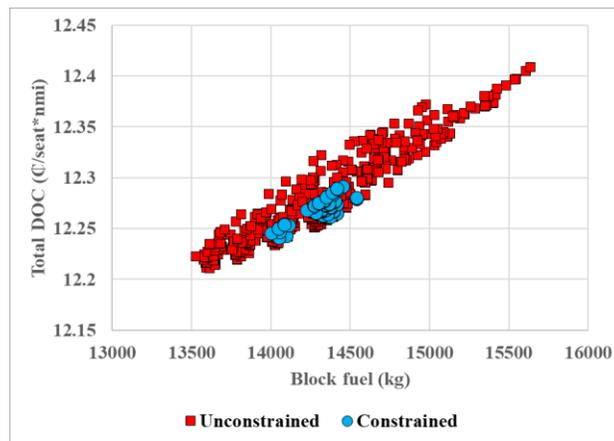
**Fig. 16 Comparison between unconstrained and constrained feasible solutions in terms of block fuel and total DOC.**
