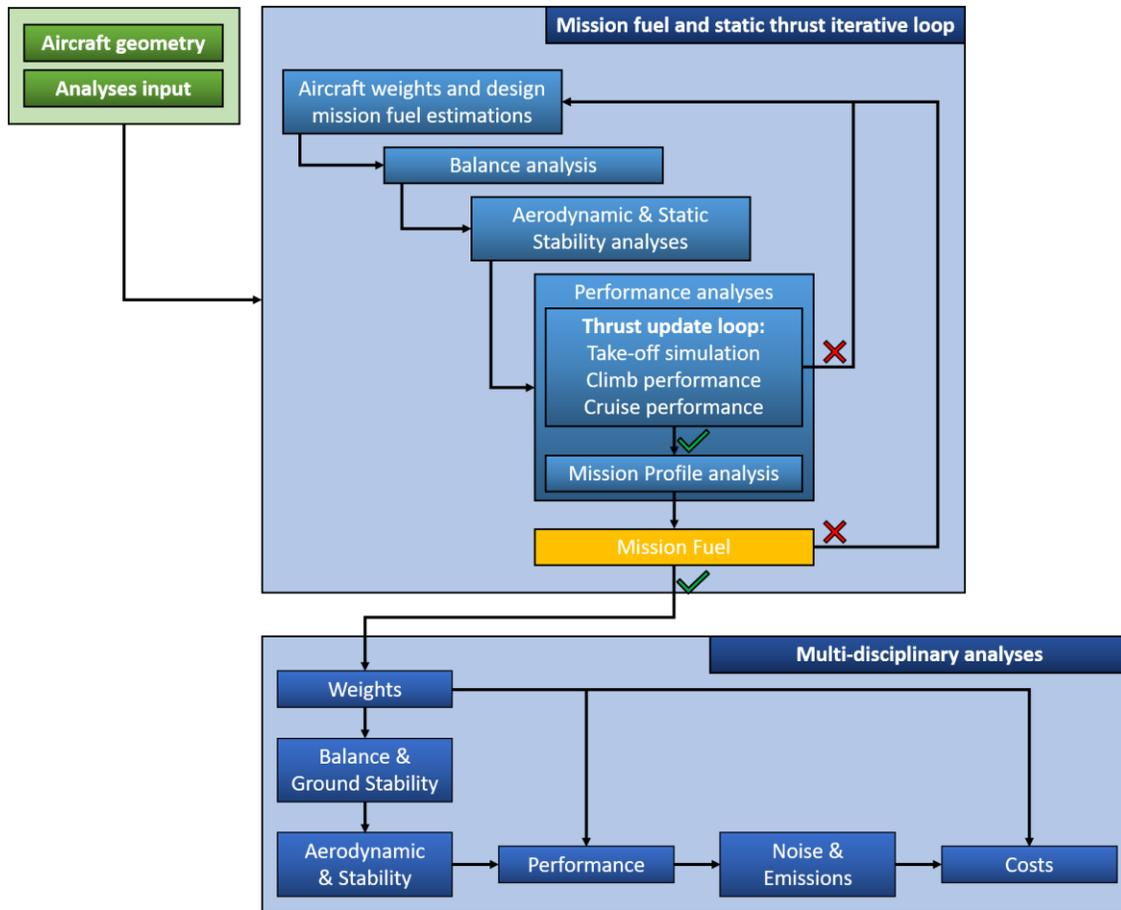
Fig. 3 JPAD complete analysis loop.
