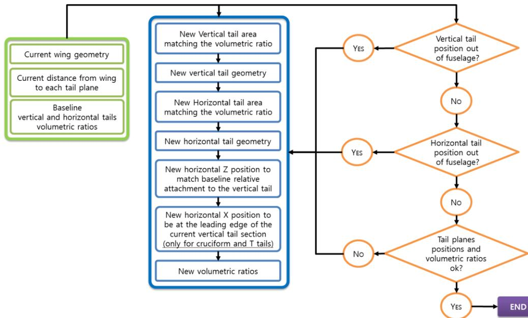
Fig. 5 Tail planes geometries and positions update loop implemented inside the JPAD DOE module.
