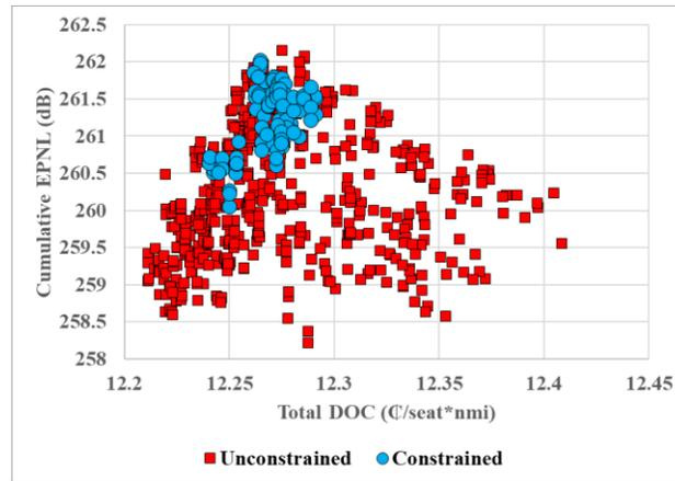
**Fig. 18 Comparison between unconstrained and constrained feasible solutions in terms of cumulative EPNL and total DOC.**
