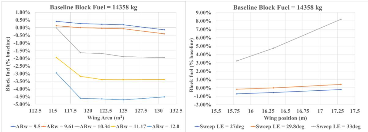
Fig. 10 Block fuel trade factors without feasibility constraints.
