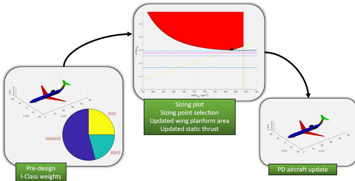
**Fig. 4 JPAD initializer complete workflow.**
