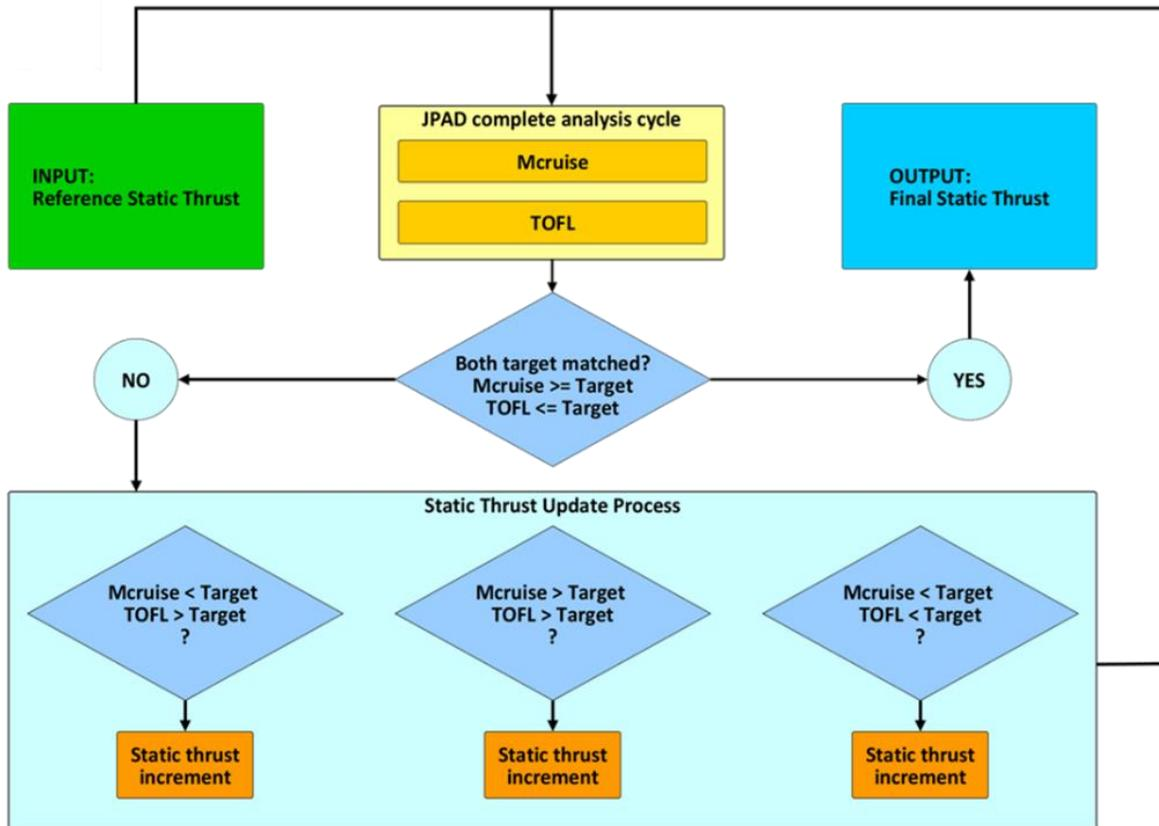
**Fig. 9 Selected static thrust update strategy for the MDA cycle of the JPAD software.**
