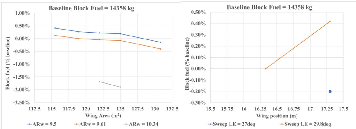
Fig. 13 Block fuel trade factors with feasibility constraints.
