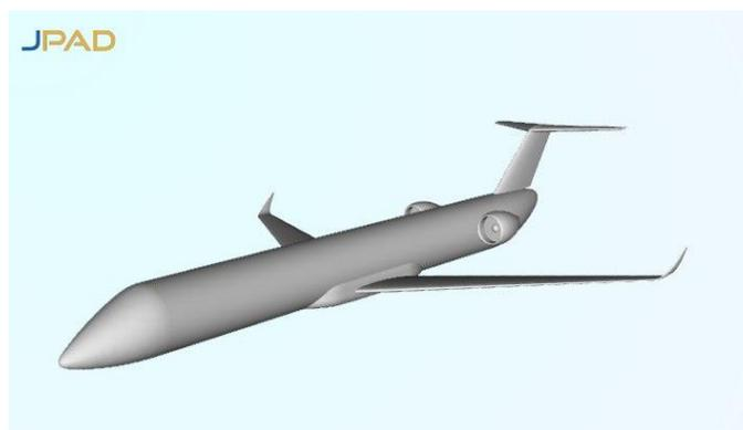
**Fig. 8 CAD model of the baseline RM A/C generated by JPAD initializer.**
