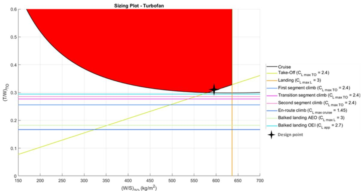
**Fig. 7 Sizing limitations, available design space and design point selection for the RM configuration.**
