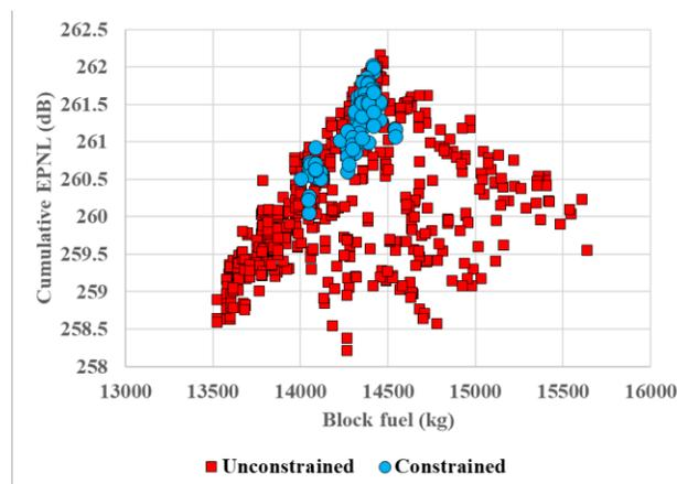
**Fig. 17 Comparison between unconstrained and constrained feasible solutions in terms of cumulative EPNL and block fuel.**
