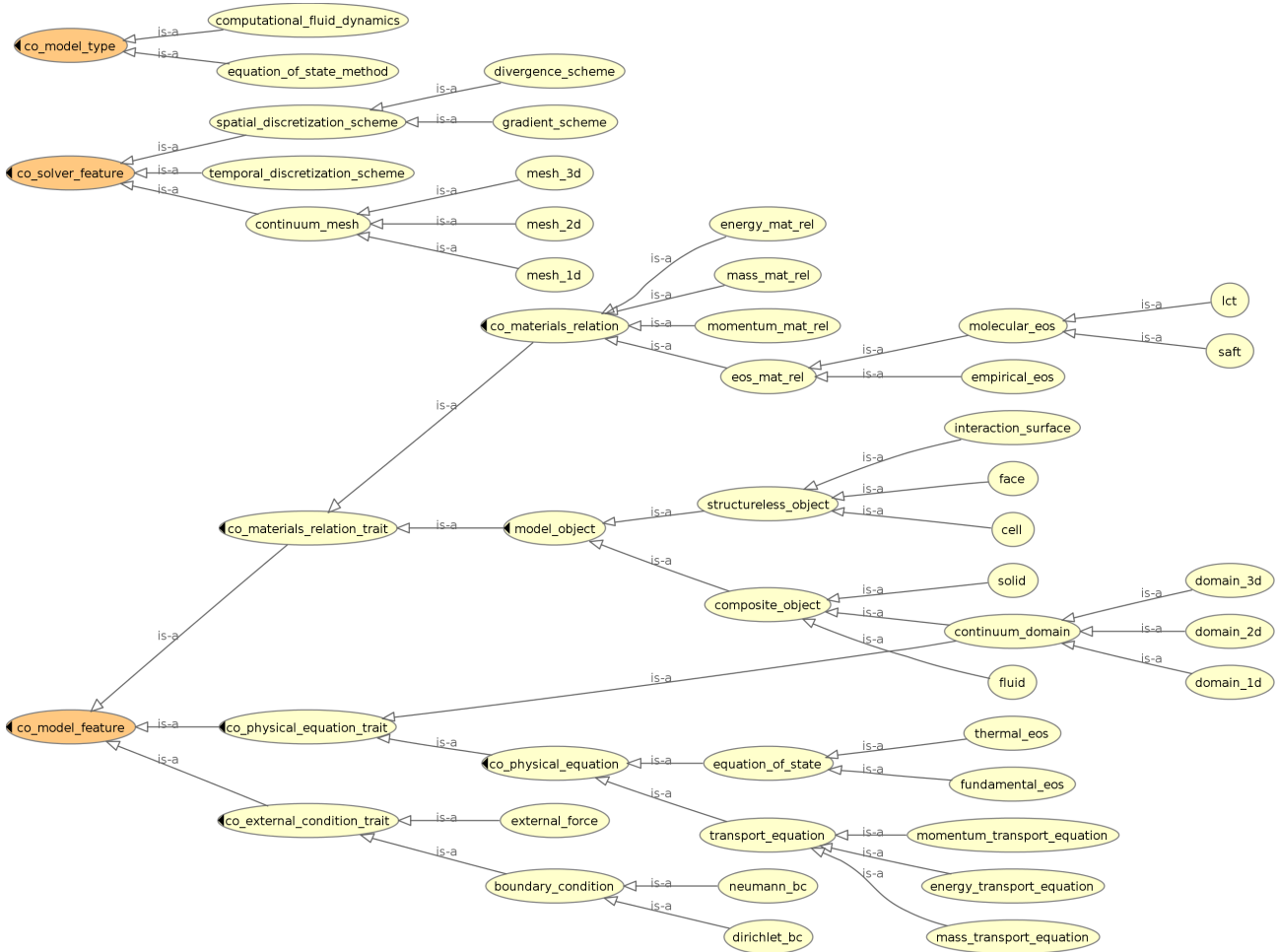
Figure 3.14. Branch of VISO for continuum models ( vivo-co ); the diagram was generated using the OWLViz protégé plugin; grey arrows labelled “is-a” denote subsumption ( \sqsubseteq ), i.e. , rdfs:subClassOf .
