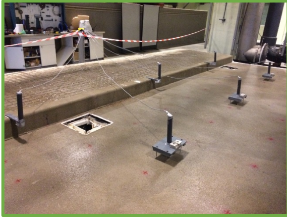
Figure 2. Distance sensors installed on the street surface (left) and on pipes (right).
