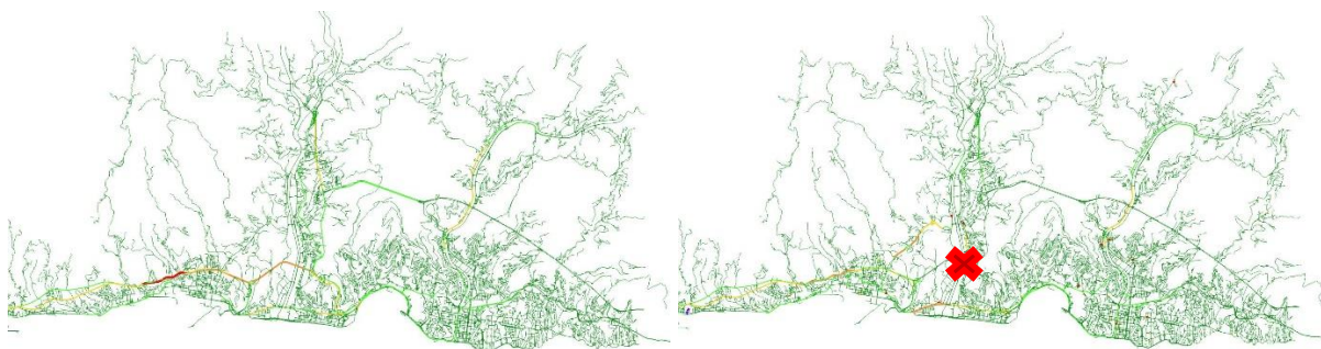
Figure 1-2: Simulation of traffic flows with Morandi bridge intact (left) and not intact (right).
