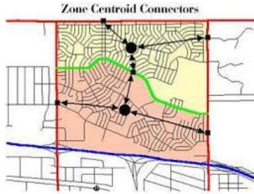
Figure 5: centroid approach for traffic generation
