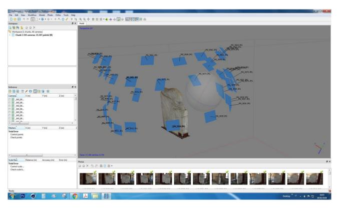
Fig. 9: 3D model from digital photogrammetry
