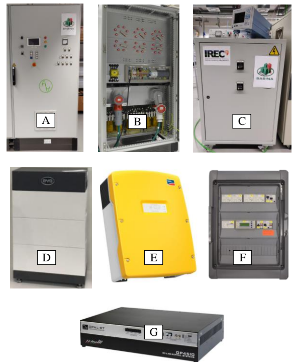
Figure 2: Some of the components of the power electronics systems, A) Grid emulator, B) Line emulator, C) Emulated load/generator, D) BYD LV lithium-ion battery, E) SMA Sunny Island inverter, F) Automatic Transfer Switch distribution panel and G) OPAL-RT simulator
