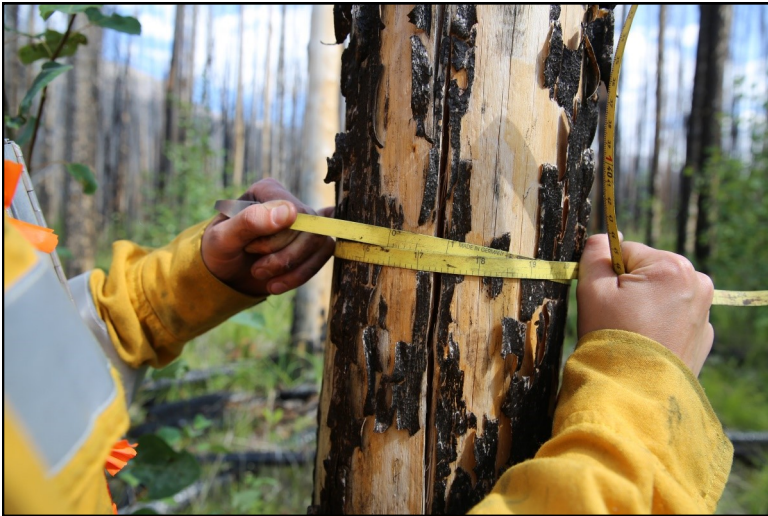
Figure 7.2 Measuring DBH on a large tree using a DBH tape. Ensure the tape is snug around the circumference of the tree.
