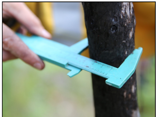
Figure 6.3 Measuring sapling DBH using a small pair of calipers at breast height.
