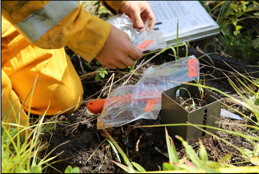
Figure 2.5 Soil core sample. Crew member has already cut and removed the soil core from the ground, and is now preparing to place the sample in a ziplock bag with its corresponding flagging tape label. In this case, mineral soil was hit less than 10cm down and thus the whole soil core cube was not filled with sample.
