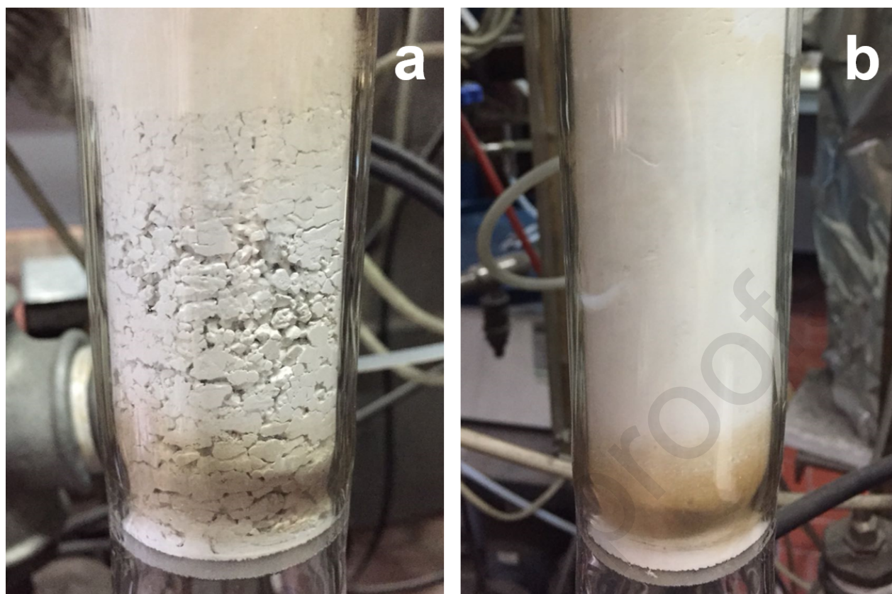
Figure 6. Pictures of the fluidized bed taken during ordinary (a) and sound-assisted (150dB – 120 Hz) (b) fluidization tests. Temperature = 850 °C.
